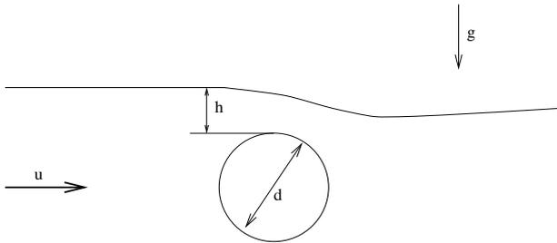
Figure 1: Schematic of the flow arrangement
