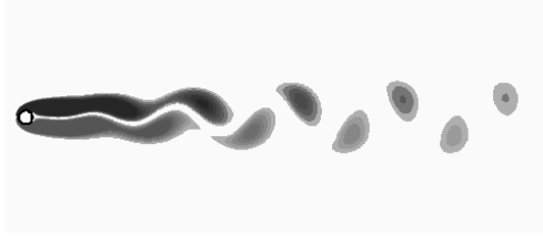
Figure 3: Vorticity field in the wake at Re = 48 .
