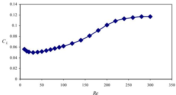
**Figure 3.** Lift coefficient for  $\Omega = 0.10$ .
