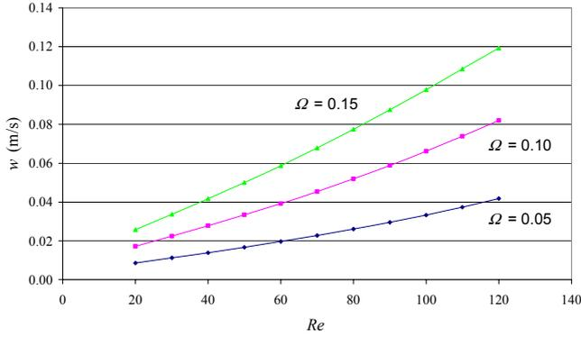
**Figure 6.** Azimuthal velocity at a location  $(x,y,z) = (4.5,0,0)$ .
