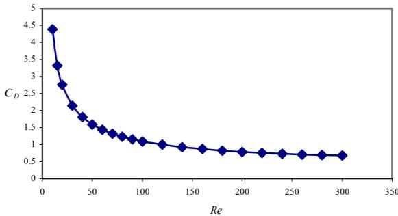
**Figure 2.** Drag coefficient for  $\Omega = 0.10$ .
