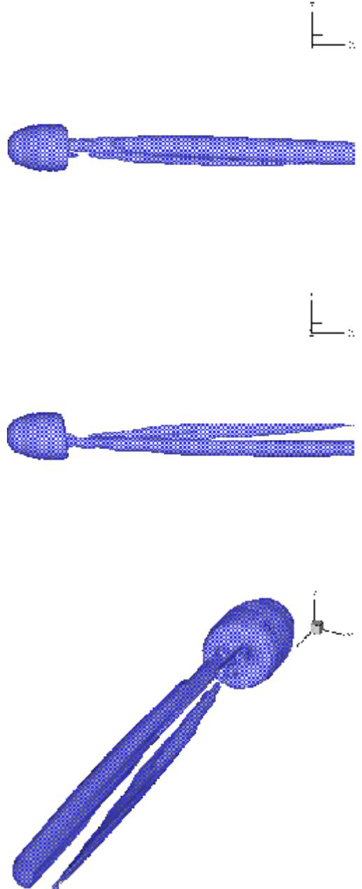
**Figure 5.** Rotating sphere about the  $x$ -axis,  $Re = 260$ .
