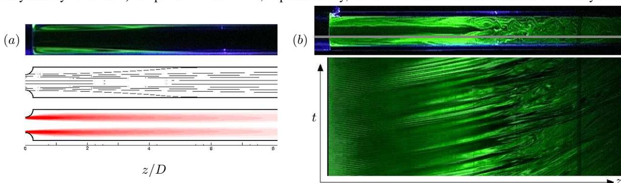
**Figure 1.** (a) Dye visualisation and numerical streamlines and vorticity for  $S = 0.75$  and  $Re = 194$ . A reflection of the laser in the middle of the image on the bottom portion of the tube is present, evident in the figure as a thin, blue shade. Flow is from left to right. (b) At top, the unsteady flow for  $S = 0.90$ ,  $Re = 194$ . For the spatio-temporal diagram, at bottom, the waves seen in the shear layer are evident as straight lines to the left of the lower diagram.
