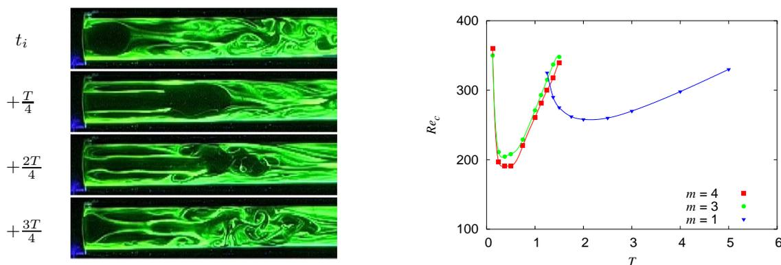
**Figure 2.** (a) Coloured-dye visualisations of the flow over one pulse period, for  $S = 0.75$ ,  $Re = 206$ ,  $A = 0.75$  and  $T = 2.43$ , (a) critical Reynolds number for linear absolute instability as a function of pulse period, for stenosis degree  $S = 0.75$ .
