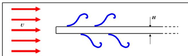
Figure 1 – Bluff plate flow geometry for numerical study.
