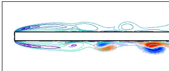
**Figure 2** – Spatial structure of dominant instability mode, from Floquet stability analysis. Red and blue indicate  $\pm$  spanwise perturbation vorticity, from -0.2 to 0.2; line contours are of spanwise vorticity, indicating positions of von Karman vortices.
