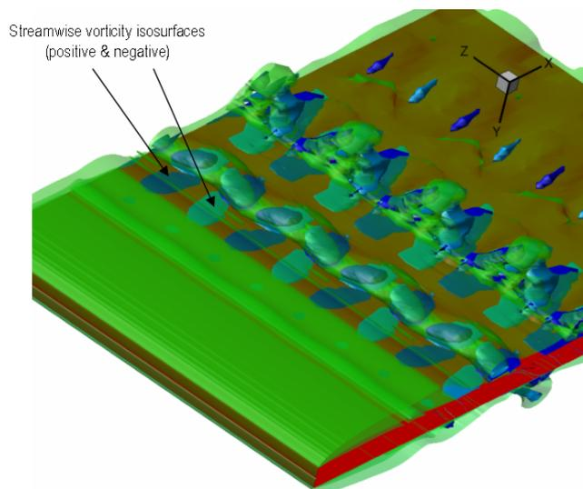
**Figure 3** – Visualisation of simulated three-dimensional flow over bluff plate (from lower left to upper right). Green and blue isosurfaces correspond to spanwise and streamwise vorticity respectively; the plate is in red.
