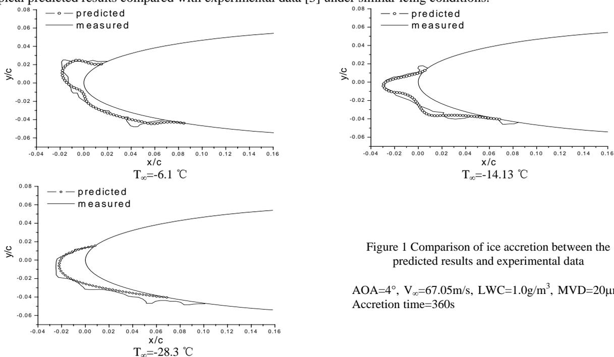
Figure 1 Comparison of ice accretion between the predicted results and experimental data
