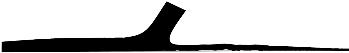
Fig. 7. Predicted flow patterns from SPH simulation at an early stage of development, of an impinging jet onto a moving surface, at Re = 50 , plate velocity (right to left) 0.5 times nozzle velocity; \theta = 30^\circ (resolution approx. 95,000 particles), Fr = 4.0 .
