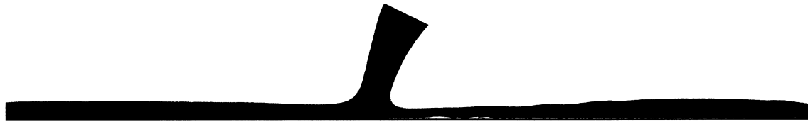
Fig. 8. Predicted flow patterns from SPH simulation at an impinging jet onto a moving surface, at Re = 50 , plate velocity (right to left) 0.5 times nozzle velocity; \theta = 30^\circ (resolution approx. 70,000 particles), Fr = 1.0 .
