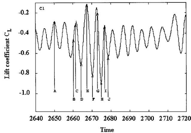
Figure 7. Close up view of the lift trace for a gap ratio of 0.40 and Froude number 0.55. (Original in colour)
