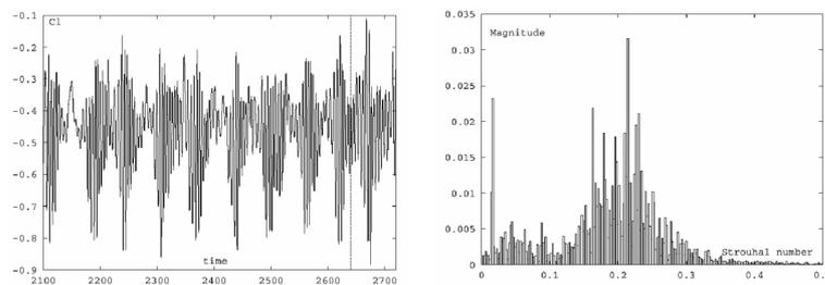
Figure 6. Lift history (left) and power spectrum (right) for a gap ratio of 0.40 and Froude number 0.55.
