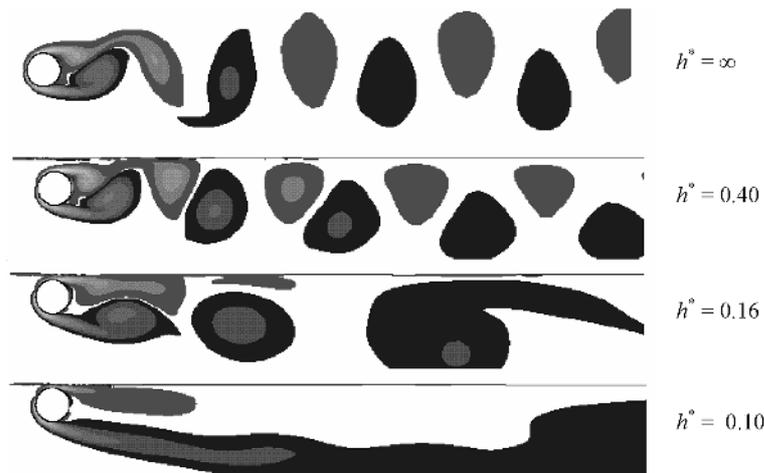
Figure 3. Vorticity plots for the reference cylinder (top) and for decreasing gap ratios,  $h^*$ , for  $Fr = 0.20$ . (Original in colour)
