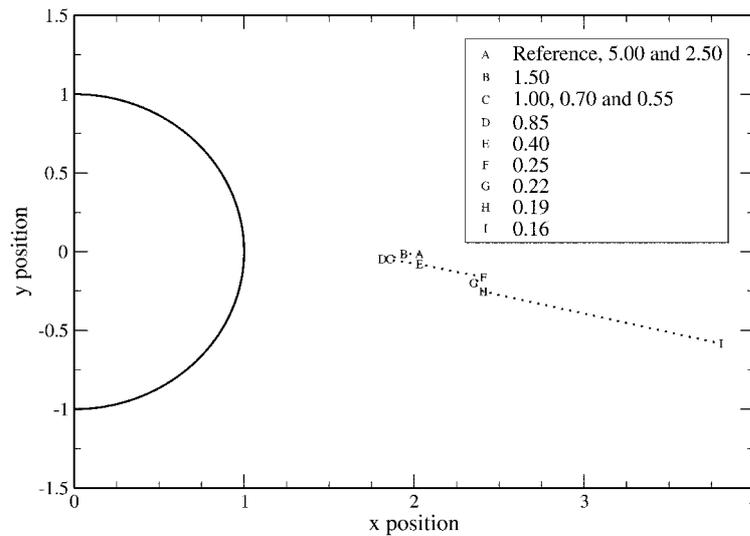
Figure 5. Position of the vortex formation position calculated using the standard deviation in the vertical velocity for a Froude number of 0.20 and different gap ratios  $h^* = h/d$ .
