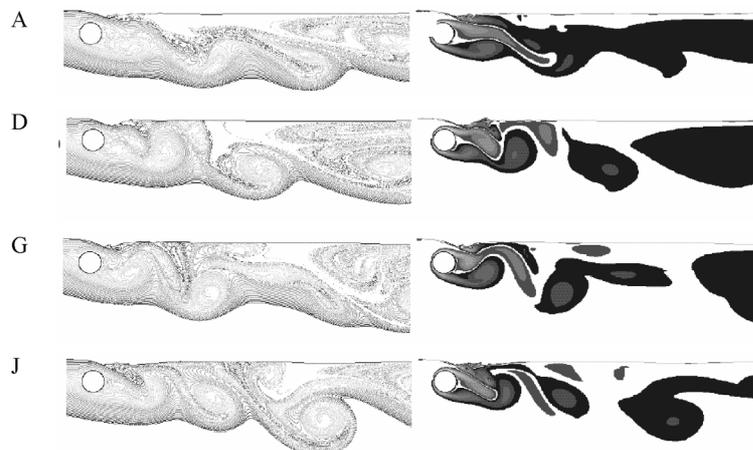
Figure 8. Passive tracer particle transport (left) and vorticity plots (right) showing flow state at some of the instants of time A-J denoted in Figure 7.
