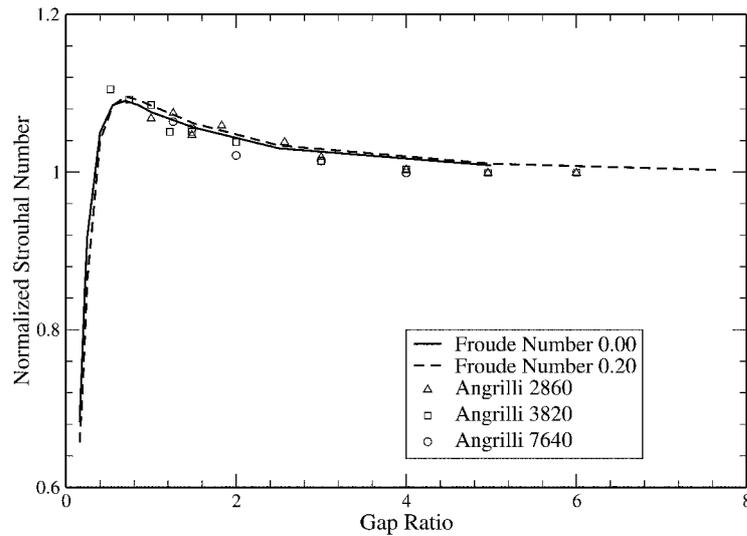
Figure 2. Variation of Strouhal number (normalized with respect to Strouhal number of the reference cylinder, i.e.  $St/St_0$ ) with gap depth  $h^*$ , for both the  $Fr = 0.00$  and  $Fr = 0.20$  cases. Also shown are the results of Angrilli et al. [1].
