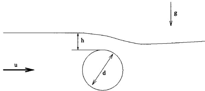
Figure 1. Schematic of the flow arrangement for a submerged cylinder.
