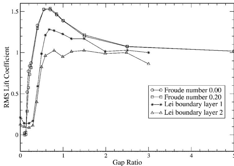
Figure 4. Plot showing the variation of RMS lift coefficient with gap ratio  $h^*$  for the free slip ( $Fr = 0.00$ ) and  $Fr = 0.20$  cases. Also plotted are the results of Lei et al. [11] (for their boundary layers 1 and 2). (Original in colour)
