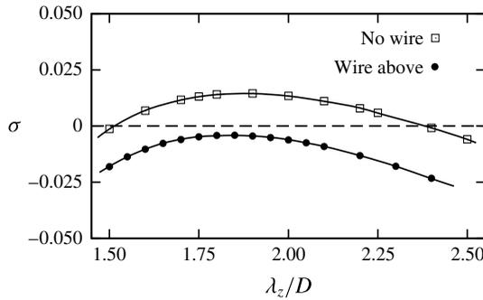
FIGURE 11. Comparison of the growth rate curves for the mode E instability at  $\alpha = 2$ ,  $Re = 220$  with the wire above the cylinder centreline ( $-\bullet-$ ) and without the wire ( $-\square-$ ). This 3D mode is stabilised by the wire, with the critical Reynolds number shifted from  $Re \simeq 207$  to  $\gtrsim 220$  at this rotation rate.
