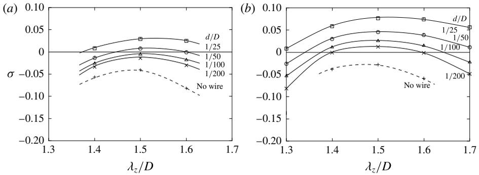
FIGURE 8. Variation of the growth rate of mode C as a function of spanwise wavelength for different wire diameters: (a)  $\alpha = 0.5$ ; (b)  $\alpha = 1.0$ . The corresponding growth rate curves for the cases without the wire are also shown, confirming mode C remains stable. Wire position  $(x, y) = (-5D, 1D)$  and  $Re = 275$ .
