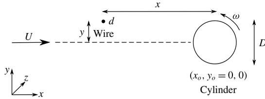
FIGURE 3. Schematic of the numerical set-up. The wire, of diameter  $d$ , is placed upstream of the rotating cylinder (diameter  $D$ ). The cylinder centreline is show by dashed lines (--).
