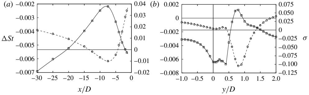
FIGURE 7. Variation of the change in Strouhal number relative to the no-wire case,  $\Delta St$  ( $\circ$ , dashed lines), and the growth rate  $\sigma$  ( $\square$ , solid lines) of the mode C instability as the wire location is varied in (a) the streamwise direction ( $x/D$ ) ( $y/D = 1$ ), and (b) the transverse direction ( $y/D$ ) ( $x/D = -5$ ) for  $\alpha = 1$ ,  $Re = 275$ .
