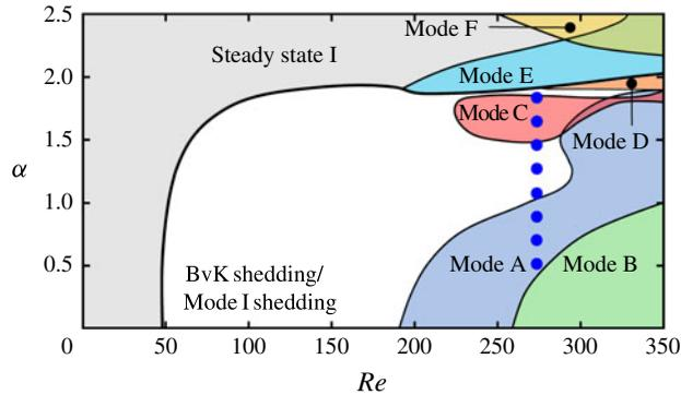
FIGURE 1.  $(Re, \alpha)$  parameter space map adapted from Rao *et al.* (2013a) showing the critical curves for flow transition from a steady or unsteady 2D base-flow state. Modes A and B correspond to the first two 3D transitions for a non-rotating cylinder. The points marked with blue circles show locations where mode C was observed in the experiments of Radi *et al.* (2013), clearly extending well below the lower boundary of the mode C C region.
