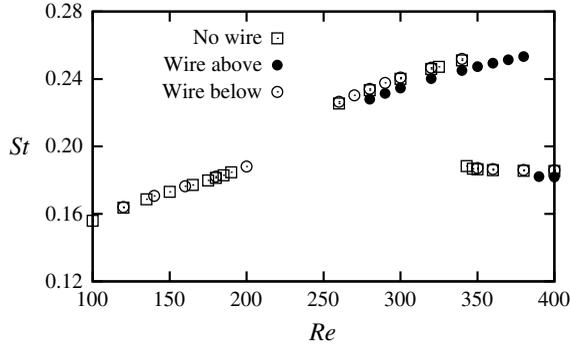
FIGURE 10. Comparison of the shedding frequencies for the rotating cylinder at  $\alpha = 1.9$ , when the wire is positioned above ( $\bullet$ ) and below ( $\circ$ ) the cylinder and the case without the wire ( $\square$ ).
