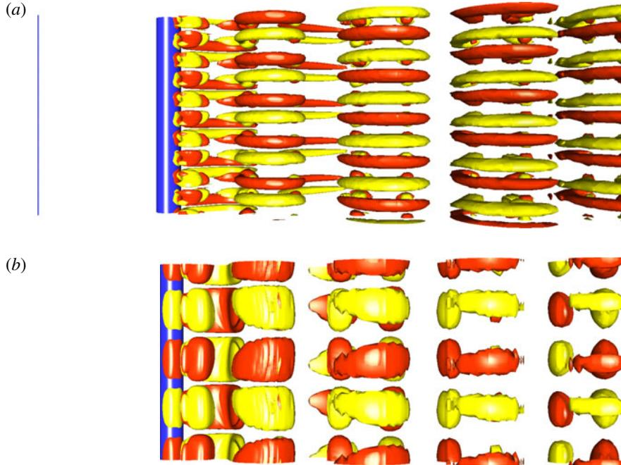
FIGURE 9. (a) Mode C (with wire); top view of streamwise vorticity isosurfaces showing saturated mode C state at  $\alpha = 1$ ,  $Re = 280$ . Flow is from left to right and the cylinder spans  $8D$ . The wire, which in this case is modelled as a cylinder of diameter  $1/25$ th  $D$ , is seen far left in this image. (b) Mode A (without wire) shows the top view of the wake without the wire for the same  $\alpha$  and  $Re$ . In this case, the flow saturates to the mode A state.
