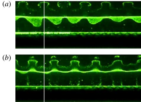
FIGURE 2. Experimental flow visualisation of the saturated mode C wake at  $\alpha = 1$ ,  $Re = 275$ . The span shown is  $\simeq 8D$ . The two images are one period apart. The white guidelines show the mushroom vortical structures are displaced by half a spanwise wavelength from one period to the next. The upstream wire is not shown. Flow is from bottom to top, with the rear of the cylinder visible at the bottom of the images. (a)  $t = t_0$ ; (b)  $t = t_0 + T$ .
