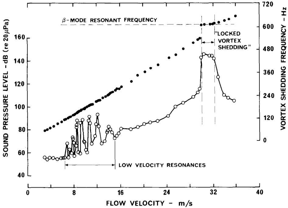
Fig. 2. Variation of vortex shedding frequency and SPL at the  $\beta$ -mode frequency with flow velocity; ●, vortex shedding frequency; ○, SPL at  $\beta$ -mode frequency.
