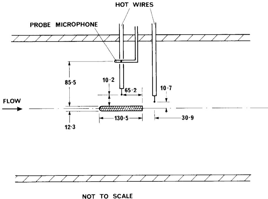
Fig. 1. Schematic of wind tunnel working section.
