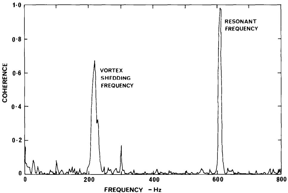
Fig. 3. Coherence of signals from the hot wire and the probe microphone located above the mid-chord position of the plate; flow velocity = 12 m/s; SPL = 93 dB.
