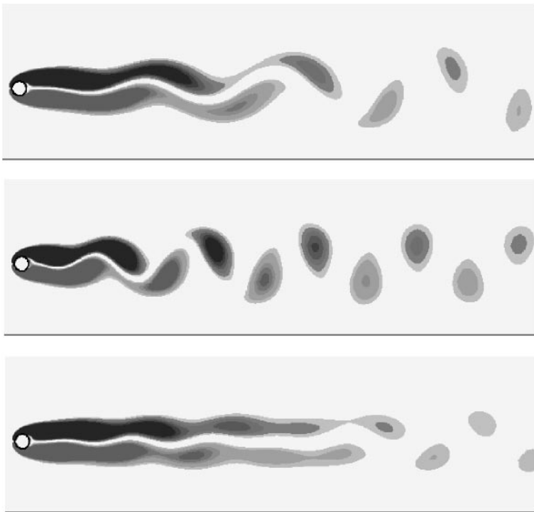
Figure 7. Vorticity plots of the oscillating wake. The forcing amplitude is set to 0.01. The centre plot shows the response at close to the optimal forcing frequency. The top and bottom plots show the wake for forcing frequencies 25% below and 25% above the resonant frequency, respectively.
