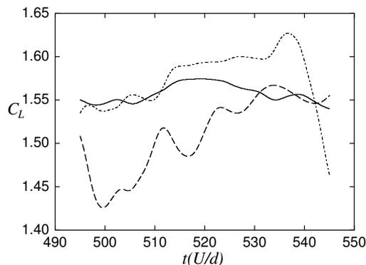
Figure 19: Evolution of the sectional lift coefficient at two spanwise locations (dashed lines) separated by half the span width at  $Re = 160$  in the fully saturated state. The spanwise averaged lift coefficient is also shown by the solid line. The period corresponding to two-dimensional vortex shedding is approximately 20 units.
