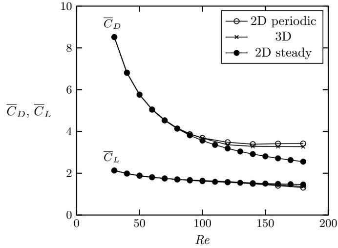
Figure 16: Comparison of time-averaged body force coefficients, drag  $\bar{C}_D$  and lift  $\bar{C}_L$ , between the two- and three-dimensional simulations for  $30 \leq Re \leq 180$ . Note that beyond  $Re_{c,2D}$  the 2D-steady predictions shown by the filled circles are based on flows calculated with the steady solver.
