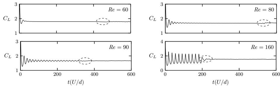
Figure 18: Temporal evolution of the lift coefficient from  $Re = 60$  to 160 computed from the three-dimensional direct numerical simulations. The dashed ellipses show the instant at which the three-dimensional instability has grown sufficiently to alter the two-dimensional flow.
