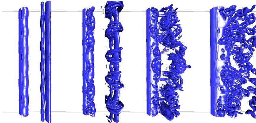
Figure 23: Stages in the evolution of the wake at  $Re = 160$  as depicted by isosurfaces of  $Q = 0.01$ . The first three images show the wake structure for three consecutive cycles just after the three-dimensionality is starting to modify the flow. The final image is a typical image after the flow has reached its asymptotic state.
