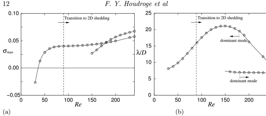
Figure 6: Left: (a) Maximum growth rate of the most unstable mode for transition from 2D steady to 3D steady flow. Right: (b) Variation of the wavelength of the fastest growing mode with the Reynolds number. Beyond  $Re \sim 150$  there are two peaks in the growth rate curve with the shorter wavelength peak developing the higher amplitude for  $Re \gtrsim 180$ .
