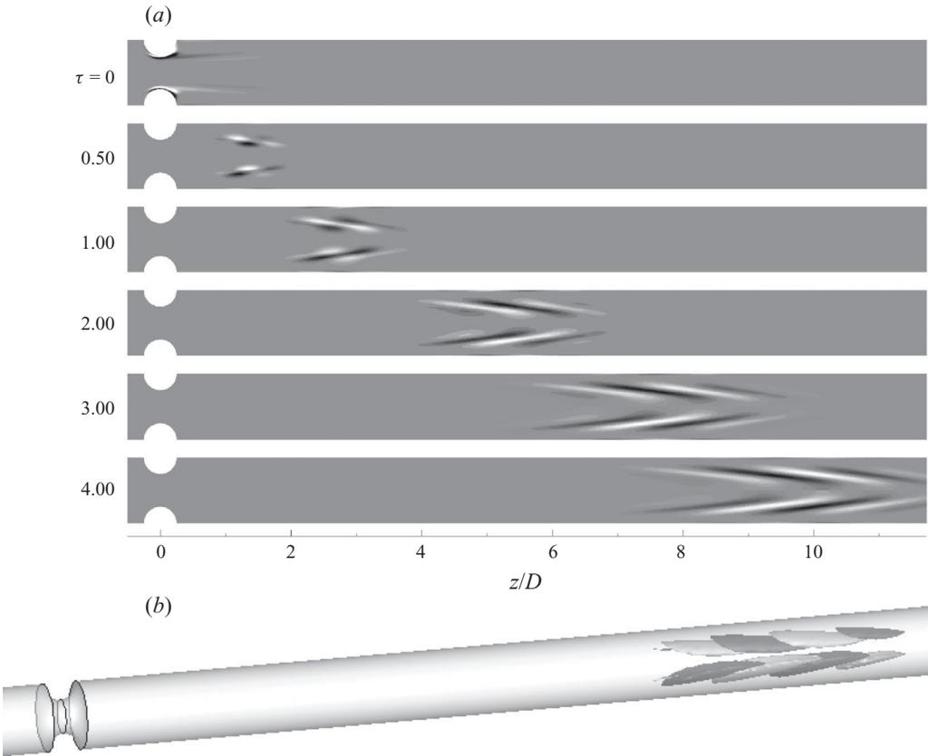
FIGURE 6. (a) Series of images of the azimuthal vorticity of the optimal disturbance for  $b = 0.75$ ,  $Re = 400$ ,  $k = 1$ , showing the development of the perturbation. Vorticity contours have been progressively enlarged in each image to show the features of the flow. (b) Three-dimensional view of the perturbation at maximal energy showing two opposite sign isosurfaces of axial vorticity. Flow is from left to right.
