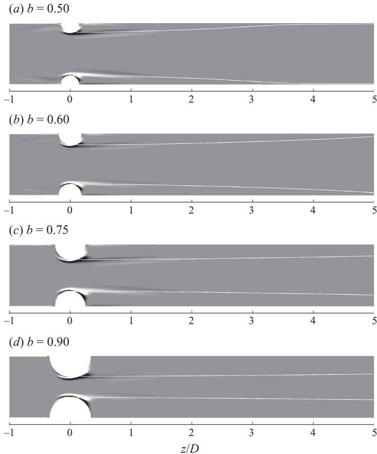
FIGURE 5. Plots of azimuthal vorticity of the optimal initial perturbation (all  $k = 1$ ) for the four different cases tested, at stenosis degrees  $b = 0.50, 0.60, 0.75$  and  $0.90$ , for the leading  $\tau$ . The separating streamline of the stable axisymmetric base flow is overlaid in each case.
