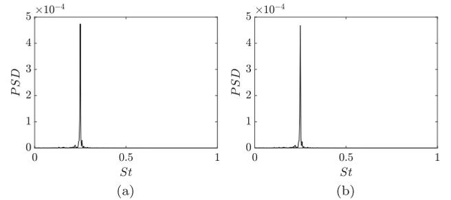
**Fig. 15.** Power spectral density of temporal content of the first two POD modes for the elliptical-nosed body, (a) Mode 1 and (b) Mode 2.
