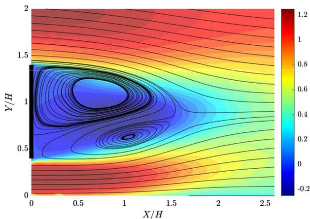
Fig. 22. Velocity profiles overlaid on contours of  $U/U_\infty$  in the near-wake of the Ahmed body cross-section for a ground clearance of  $0.4H$ .
