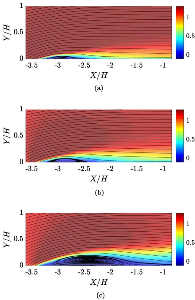
Fig. 19. Velocity streamlines superimposed on contours of  $U/U_\infty$  above the Ahmed body cross-section for (a)  $Re = 5 \times 10^3$ , (b)  $Re = 1 \times 10^4$  and (c)  $Re = 2 \times 10^4$ .
