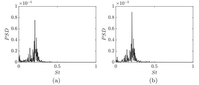
**Fig. 14.** Power spectral density of temporal content of the first two POD modes for the Ahmed body cross-section, (a) Mode 1 and (b) Mode 2.
