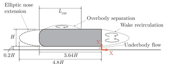
Fig. 3. Diagram highlighting key dimensions and flow features for the Ahmed-body cross-section for the  $0.2H$  ground clearance case.
