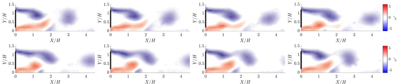
**Fig. 13.** Full cycle of phase-averaged vorticity contours in the wake of the elliptical-nosed body at  $Re = 2 \times 10^4$ , where  $\omega^*$  is defined as the vorticity, normalised based on the body height and freestream velocity.
