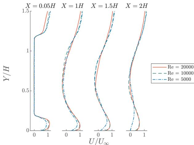
Fig. 20. Velocity profiles taken at different streamwise positions downstream of the Ahmed body cross-section.
