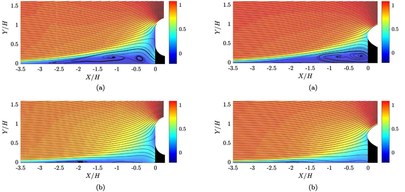
Fig. 17. Contours of  $U/U_\infty$  upstream of the model nose for the Ahmed body cross-section with overlaid streamlines for (a)  $Re = 5 \times 10^3$  and (b)  $Re = 1 \times 10^4$ . Origin taken along ground plane at model nose position.
