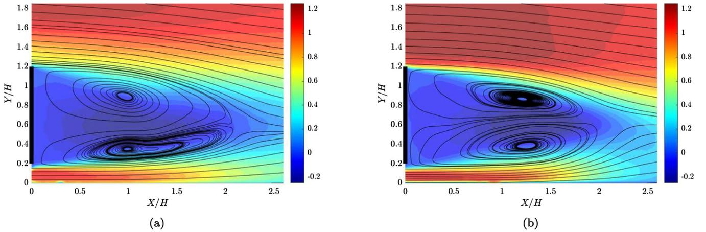
Fig. 6. Velocity profiles overlaid on contours of  $U/U_\infty$  in the near-wake of (a) the Ahmed body cross-section and (b) the elliptical-nosed body.
