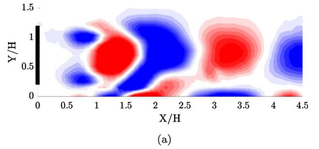
Fig. 11. First two vorticity modes for the elliptical-nosed body wake. The contours visualize the relative strength, with red signifying values above a positive threshold and blue, below a negative threshold. (For interpretation of the references to color in this figure legend, the reader is referred to the web version of this article.)
