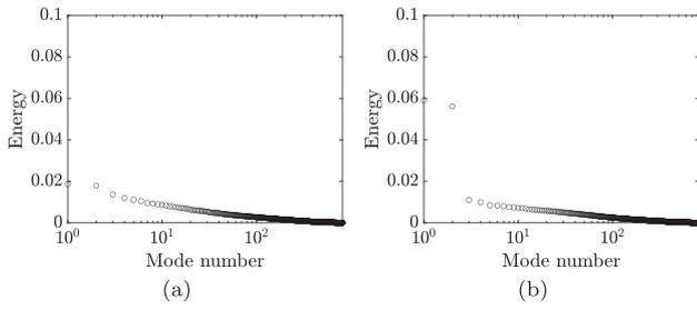
Fig. 9. Relative POD modal energy for (a) Ahmed body cross-section and (b) elliptical-nosed body.
