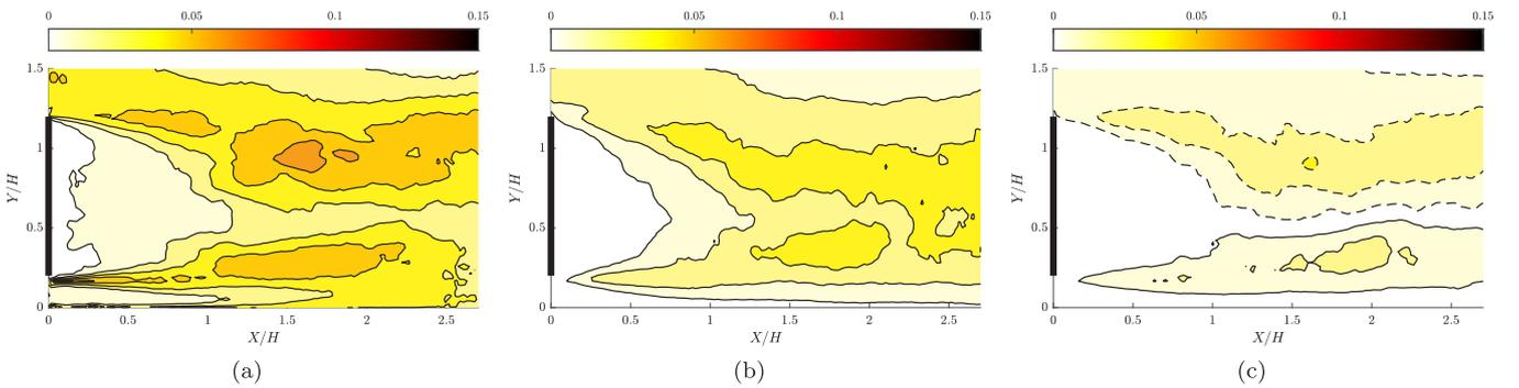
Fig. 7. Contours of Reynolds stress magnitudes in the wake of the Ahmed body cross-section. (a)  $\overline{u'u'}/U_\infty^2$ , (b)  $\overline{v'v'}/U_\infty^2$  and (c)  $\overline{u'v'}/U_\infty^2$ . Dashed lines represent negative values.
