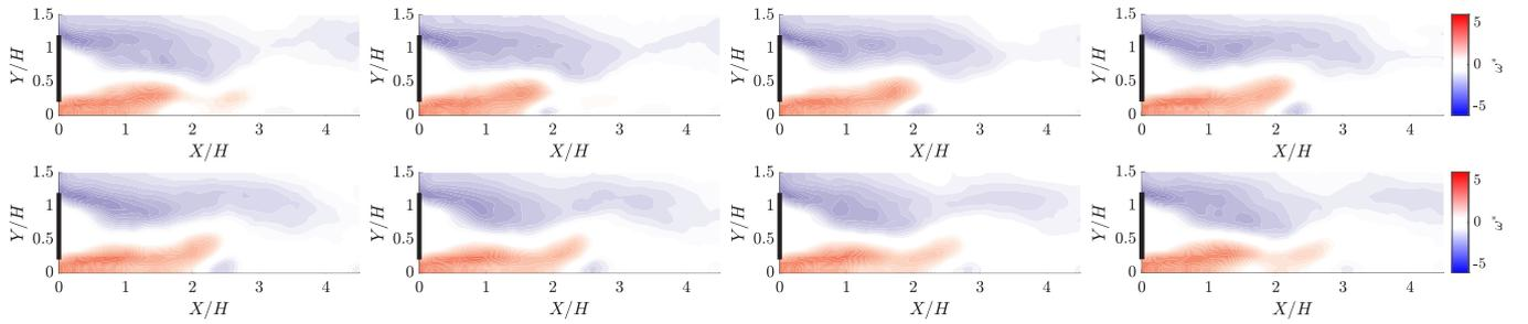
**Fig. 12.** Full cycle of phase-averaged vorticity contours in the wake of the Ahmed-body cross-section at  $Re = 2 \times 10^4$ , where  $\omega^*$  is defined as the vorticity, normalised based on the body height and freestream velocity.
