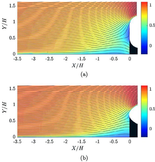
**Fig. 4.** Contours of  $U/U_\infty$  upstream of the model nose for the (a) Ahmed body cross-section and (b) elliptical-nosed body with overlaid streamlines. Origin taken along ground plane at model nose position.
