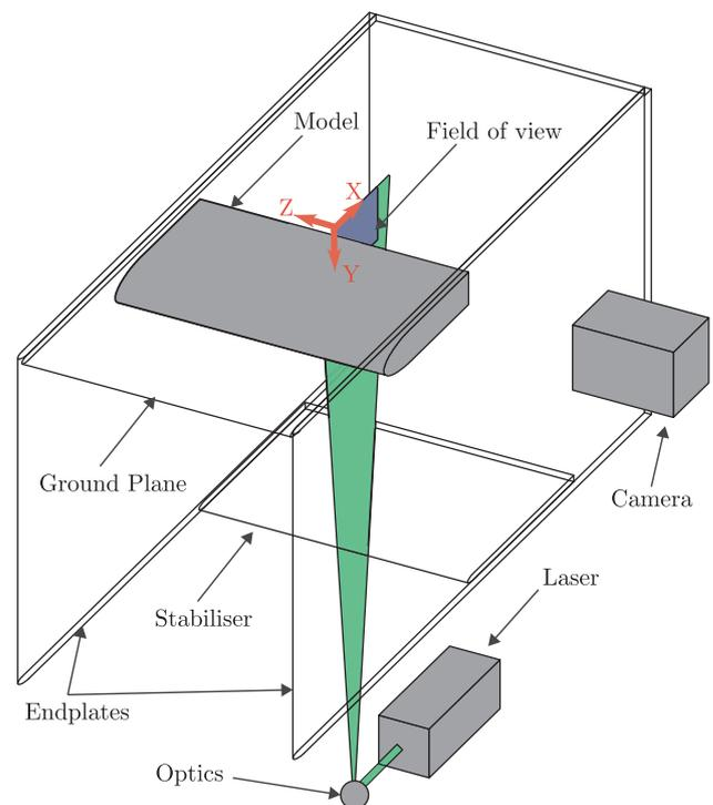
Fig. 1. Diagram of the layout of the experimental setup for capturing snapshots of the wake behind the elliptical-nosed body. The X-directional positions of the laser and camera were varied for other fields of view.
