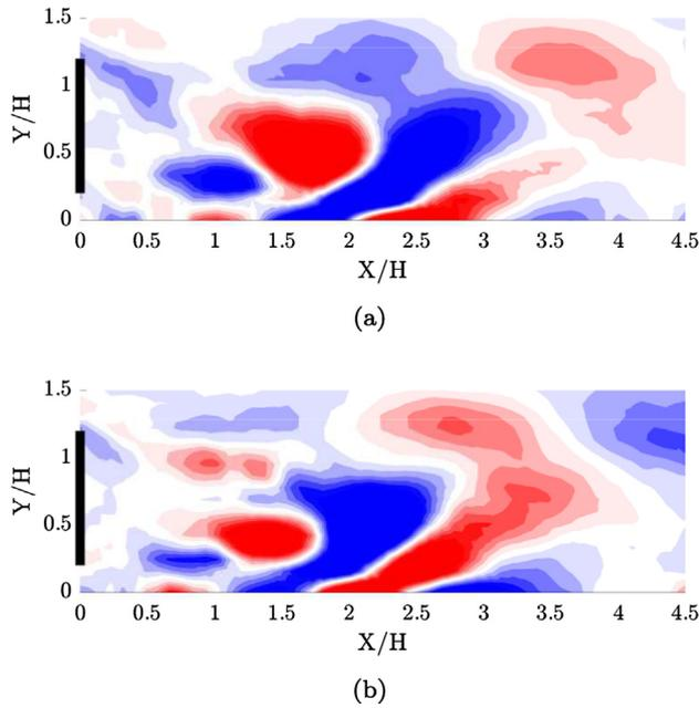
Fig. 10. First two vorticity modes for the Ahmed body cross-section. The contours visualize the relative strength, with red signifying values above a positive threshold and blue, below a negative threshold. (For interpretation of the references to color in this figure legend, the reader is referred to the web version of this article.)
