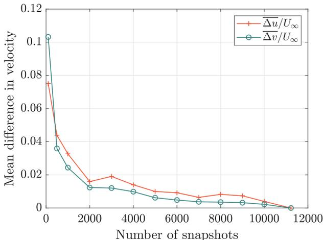
Fig. 2. Convergence of mean difference in time-averaged velocity for increasing number of image pairs relative to values using all image pairs.
