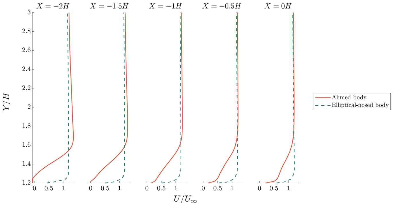
**Fig. 5.** Velocity profiles above both bodies at various streamwise positions.
