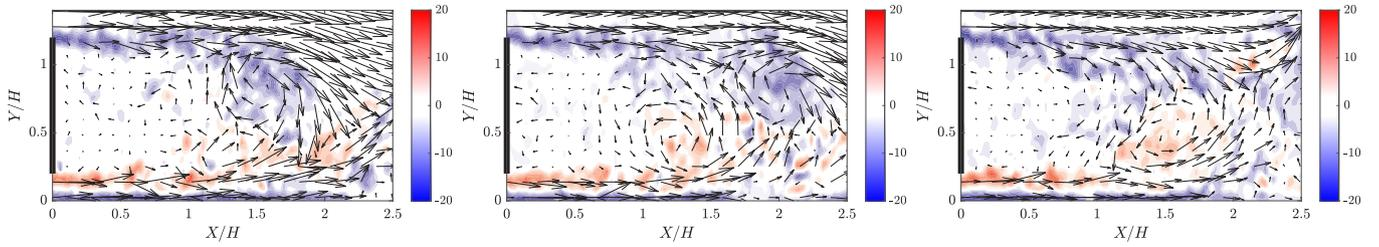
Fig. 16. Instantaneous velocity vectors in the wake of the elliptical-nosed body superimposed on contours of instantaneous vorticity highlighting different stages of the vortex shedding process over a single cycle. Snapshots taken at intervals of  $0.25 \times$  shedding period. Only every fourth vector is plotted for clarity.
