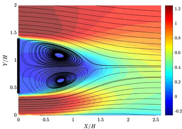
Fig. 23. Velocity profiles overlaid on contours of  $U/U_\infty$  in the near-wake of the elliptical nosed body for a ground clearance of  $0.4H$ .
