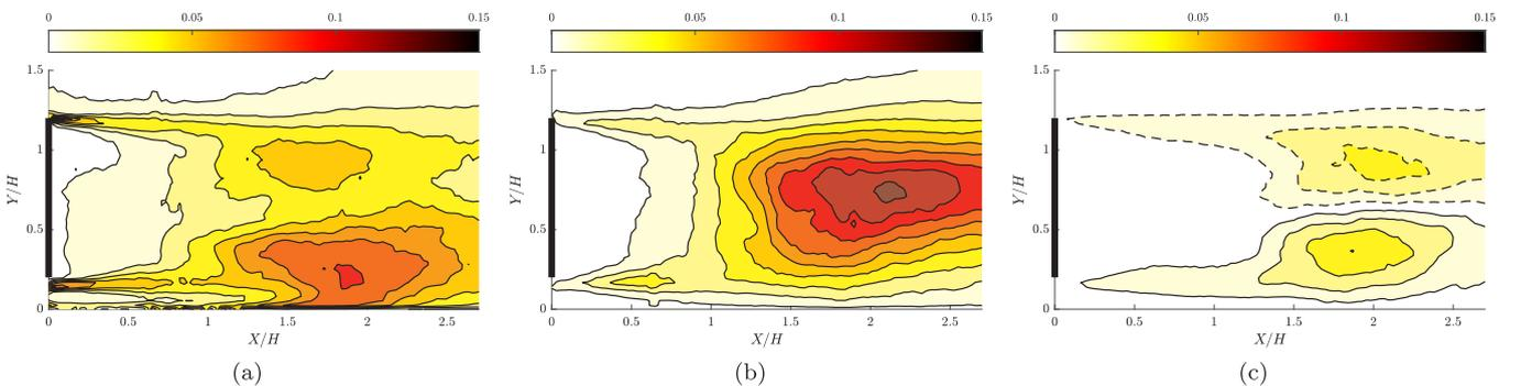
Fig. 8. Contours of Reynolds stress magnitudes in the wake of the elliptical-nosed body. (a)  $\overline{u'u'}/U_\infty^2$ , (b)  $\overline{v'v'}/U_\infty^2$  and (c)  $\overline{u'v'}/U_\infty^2$ . Dashed lines represent negative values.
