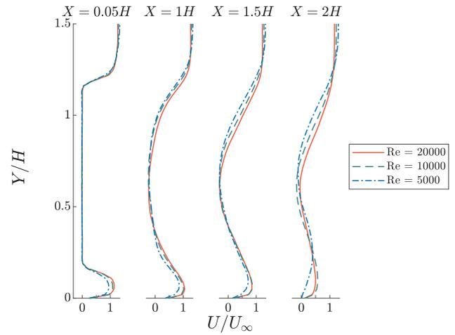
Fig. 21. Velocity profiles taken at different streamwise positions downstream of the elliptical-nosed body.
