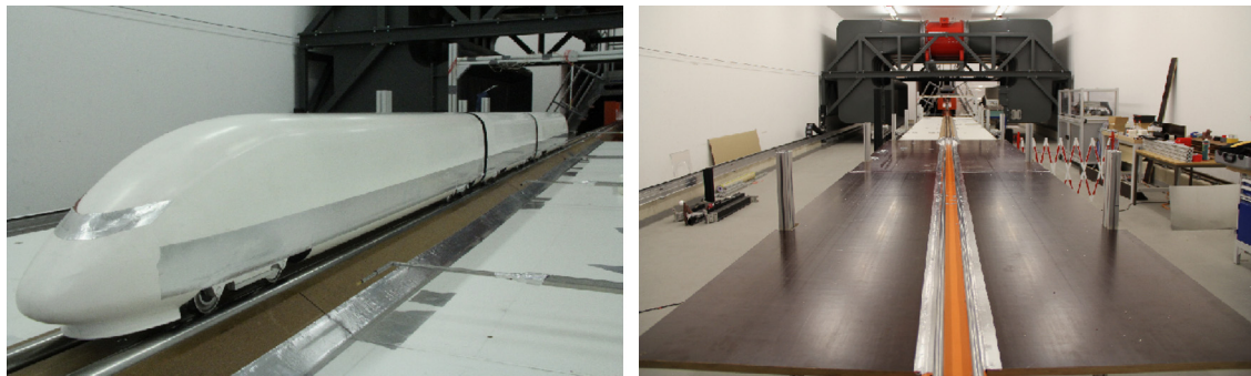
Fig. 3. Moving model experimental set-up at DLR, Göttingen.
