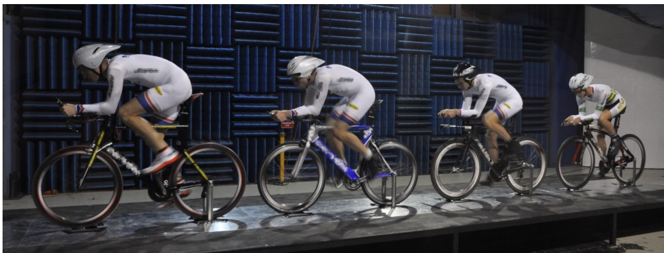
Fig. 1 Team formation on rig in wind tunnel test section (displaying Sequence 1 in descending size order)
