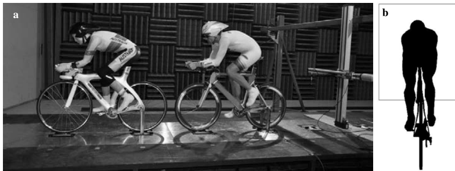
Fig. 1 – (a) Mannequin and athlete in tandem formation showing pressure probe and traverse in wake. (b) Interrogation window behind athlete.
