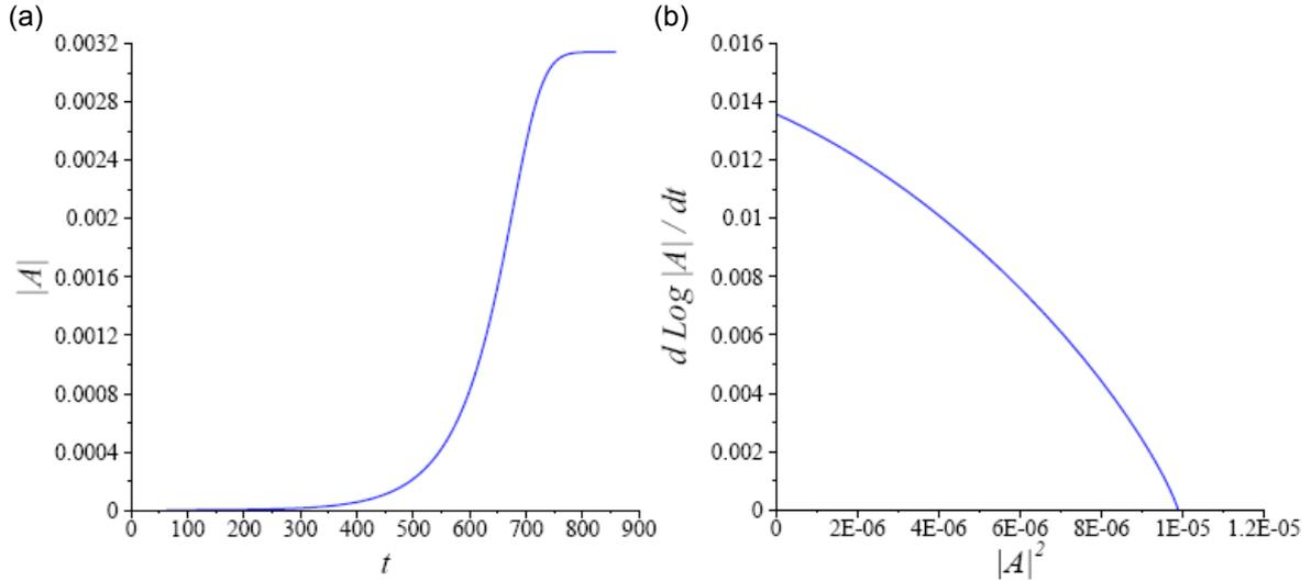
FIGURE 1: (a) The time history of an integrated amplitude norm of the Mode C instability behind a ring with  $AR = 10$  at  $Re = 170$ , with azimuthal wavelength  $\lambda_d = 1.7$ . (b) A plot of  $d(\log|A|)/dt$  against  $|A|^2$  where the negative slope at the  $y$ -axis intercept indicates that the transition is supercritical.
