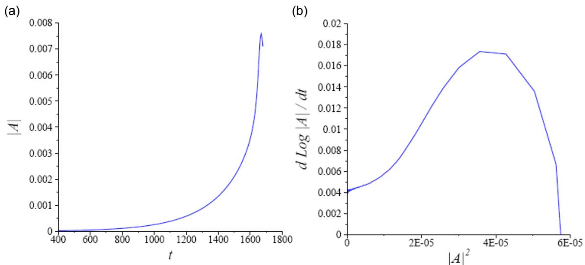
FIGURE 2: (a) The time history of an integrated amplitude norm of the Mode C instability behind a ring with  $AR = 10$  at  $Re = 230$ , with azimuthal wavelength  $\lambda_d = 1.7$ . (b) A plot of  $d(\log|A|)/dt$  against  $|A|^2$  where the negative slope at the  $y$ -axis intercept indicates that the transition is supercritical.
