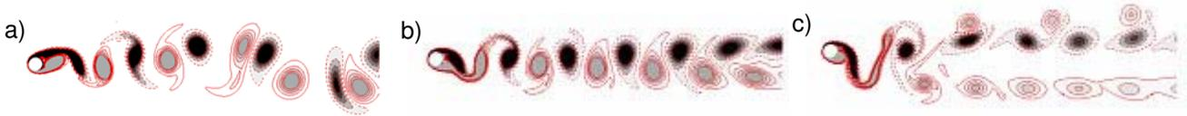
Figure 2. Vorticity contours for a) the unstable wake at  $V_r=3$ ,  $A/D=0.179$  showing low frequency modulation, b) synchronised 2S or Kármán street wake at  $V_r=5$ ,  $A/D=0.199$ . and c) the synchronised, asymmetric P+S shedding mode at  $V_r=5$ ,  $A/D=0.696$
