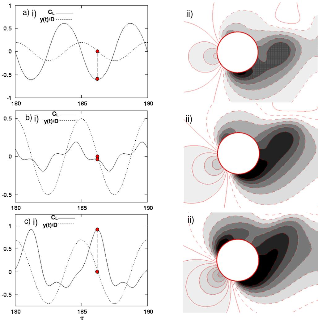
Figure 3. Lift coefficients and corresponding pressure contours for cylinder oscillating at  $V_r=5.0$ , a)  $A/D=0.199$ , b)  $A/D=0.497$  and c)  $A/D=0.696$ . Red dots indicate point at which images were obtained. Negative pressure is shown in black and enclosed by dashed contours.
