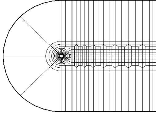
Figure 1. Macro-element mesh used during investigation.
