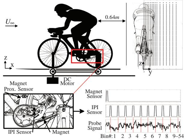
Figure 2. Side view of the setup of the pedalling mannequin. The rear view of the mannequin shows the velocity field measurement locations made in a plane a torso length (640 mm) behind the mannequin. The zoomed image of the crank shows the positioning of sensors used to determine the angle of the crank. This is shown along with an example of the phase-averaging process of probe data using signals output by these sensors. (Note: only the first 9 bins of a pedal stroke are shown for clarity).
