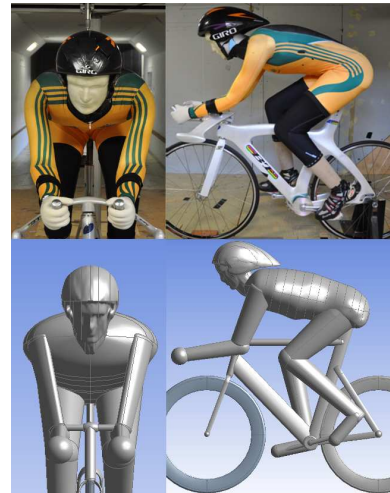
Figure 1: The two cyclist models employed. At top, the mannequin used in the wind tunnel experiments, and at bottom a sketch of the cyclist model used in the numerical simulations.
