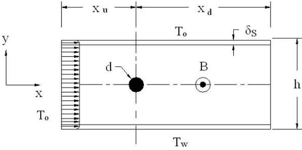
Figure 1: Schematic representation of the computational domain for the flow past a confined circular cylinder in the average plane.  $\delta_s$  is the thickness of Sherclif's layer, and  $h$  and  $d$  are respectively, the duct width and cylinder diameter.
