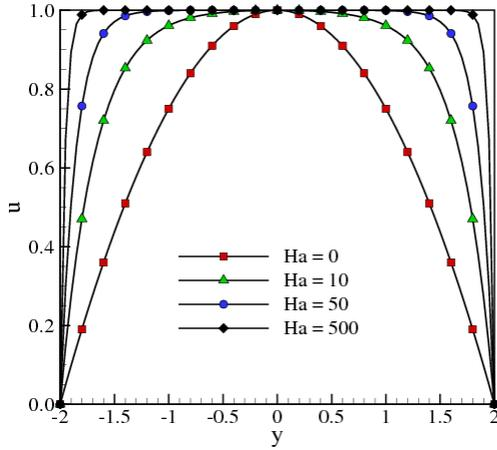
Figure 2: Base flow velocity profile at different values of Hartmann number.
