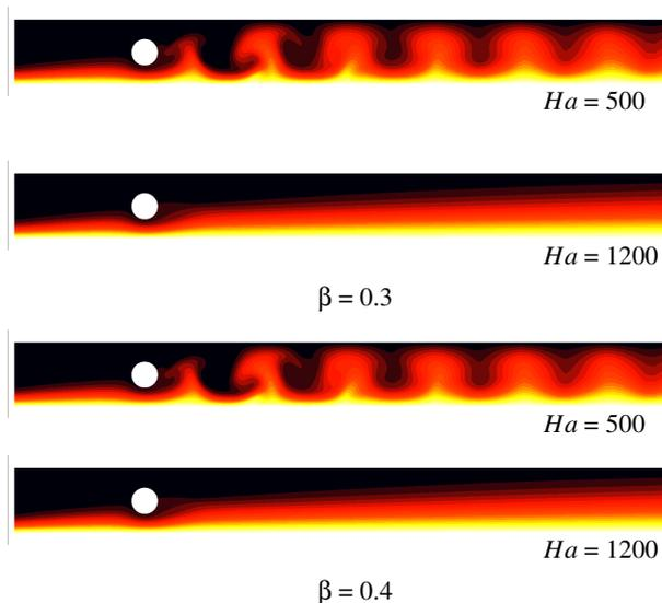
Figure 7: Instantaneous dimensionless temperature contours at  $Re = 2000$  for  $\beta = 0.3$  and  $\beta = 0.4$  at low and high Hartmann number. 20 contour level are displayed between  $0.05 \leq T \leq 0.95$ , with red and black contours representing warmer and colder temperatures respectively.
