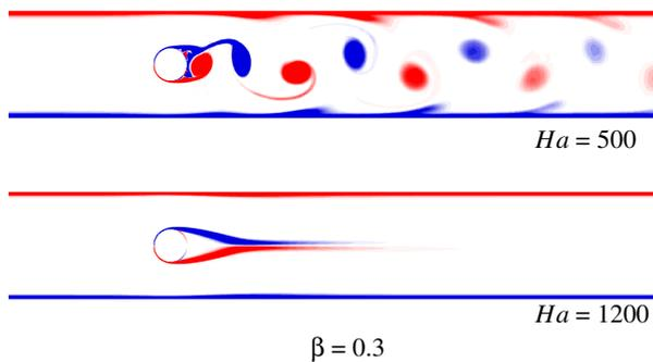
Figure 6: Vorticity contour plots for  $Re = 2000$  and  $\beta$  of 0.3 at low and high Hartmann number. 20 contour level are displayed between  $-2 \leq \omega \leq 2$ , with red and blue contours representing negative and positive vorticity.
