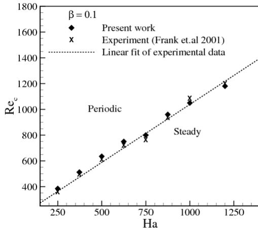
Figure 3: Comparison of critical Reynolds for the transition from steady to periodic flow with the results from other studies at different Hartmann number for a blockage ratio of 0.1.
