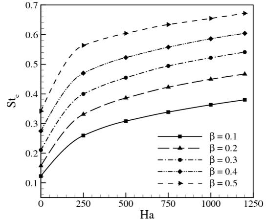
Figure 5: Variation of critical Strouhal number with Hartmann number at blockage ratio as indicated.
