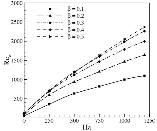
Figure 4: Variation of critical Reynolds number for the transition from steady to periodic flow with Hartmann number at blockage ratio as indicated.
