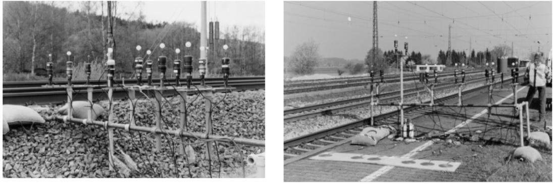
FIGURE 1.7: An example of full-scale set-up to measure the slipstream velocity at trackside (left) and on a platform (right) (Sterling et al. 2008).
