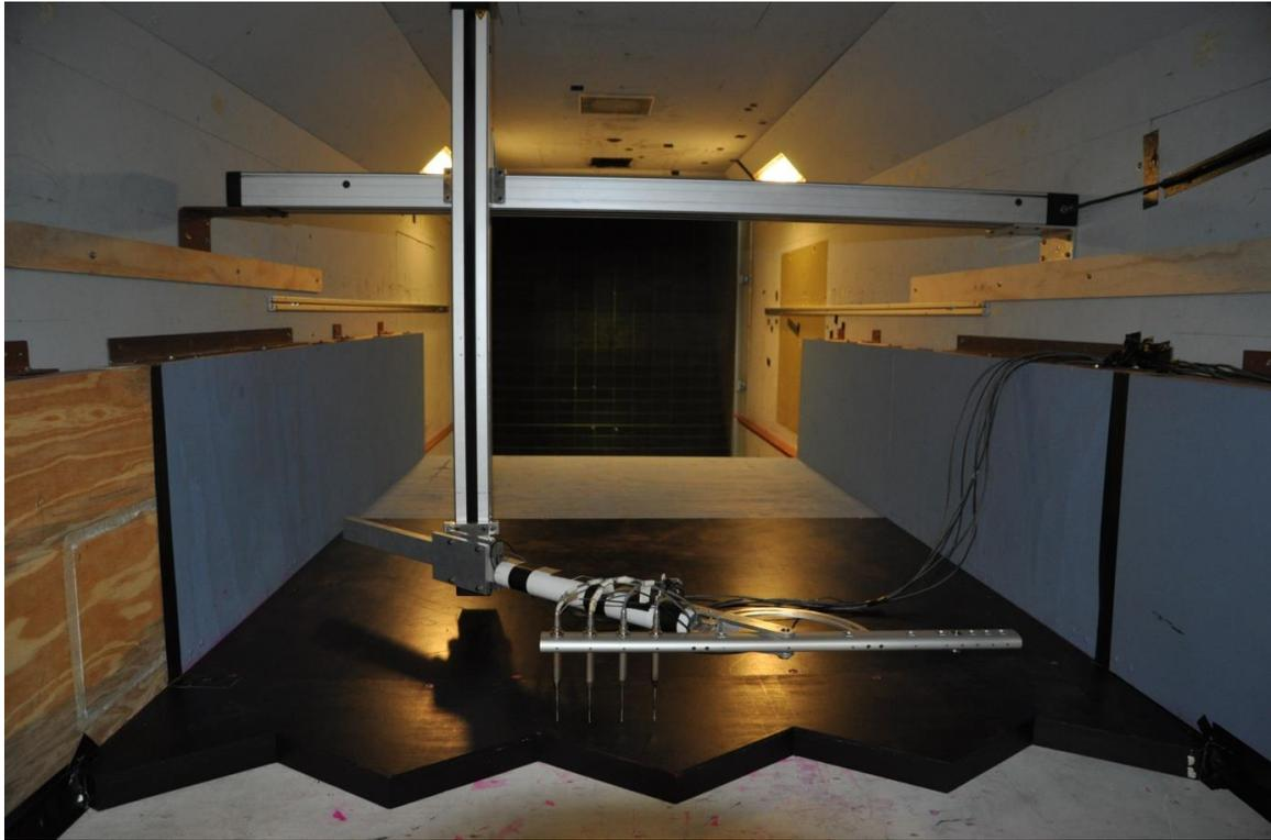
**Figure 25: Sawtooth model,  $A/\lambda = 0.325$ , shown with two-dimensional traversing equipment and four-Cobra Probe configuration.**
