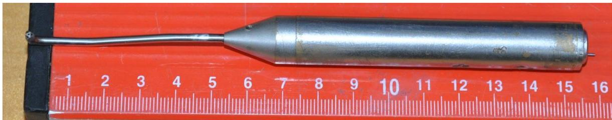
Figure 19: TFI Cobra Probe over a ruler. Units in centimetres.
