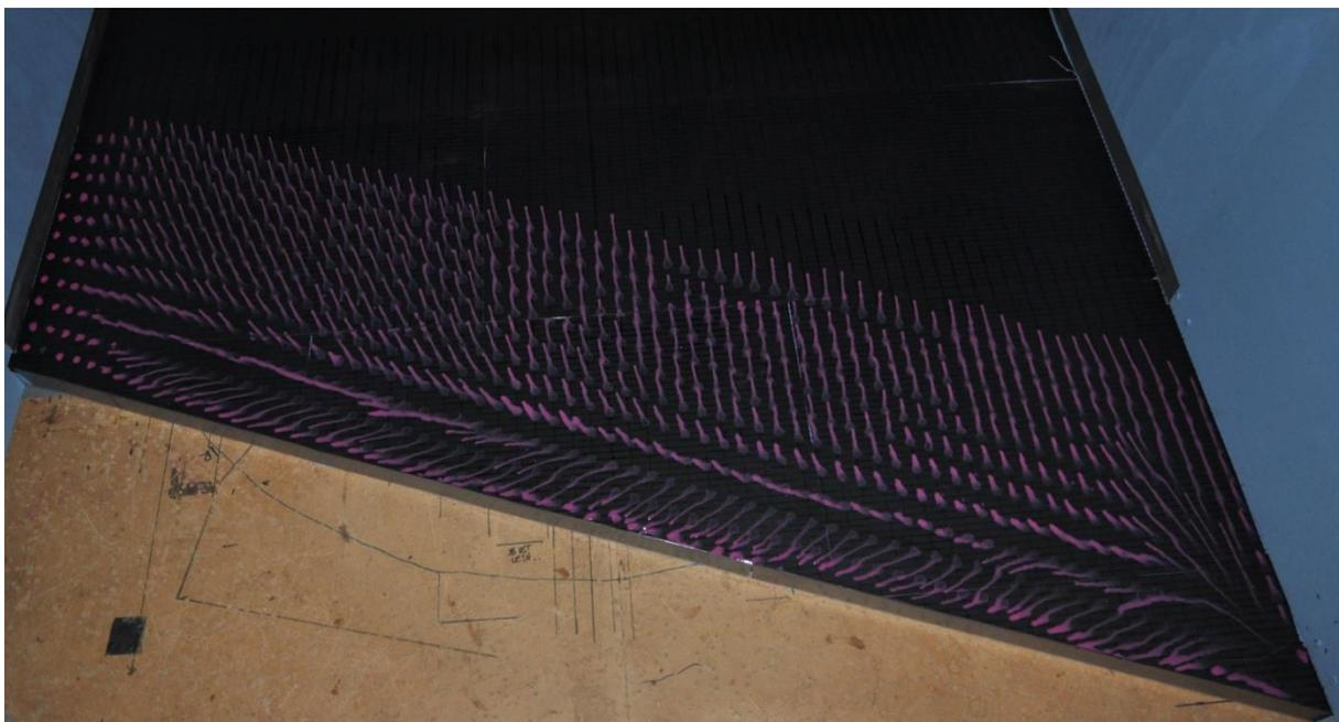
Figure 167: Paint droplet surface shear stress visualisation for  $\delta/h = 14.3$ . Yaw angle,  $\theta = 20^\circ$ . Inflow Configuration 2. Step height,  $h = 50$  mm. Flow direction from bottom of page to top.
