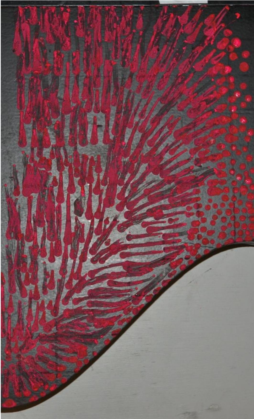
Figure 136: Surface shear stress visualisation over Sinusoidal FFS:  $A/\lambda = 0.325$ .
