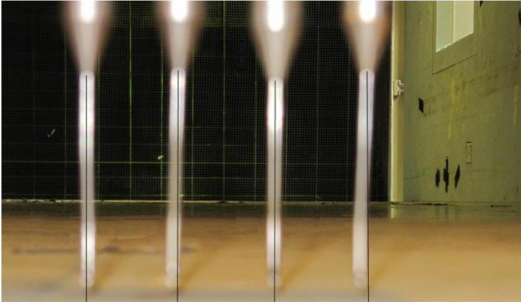
Figure 27: Slight skew of Cobra Probes with superimposed vertical lines.
