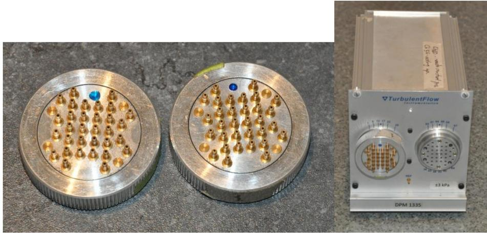
Figure 40: Manifolds for the DPMS (Left) and one DPMS unit with an attached manifold (Right).
