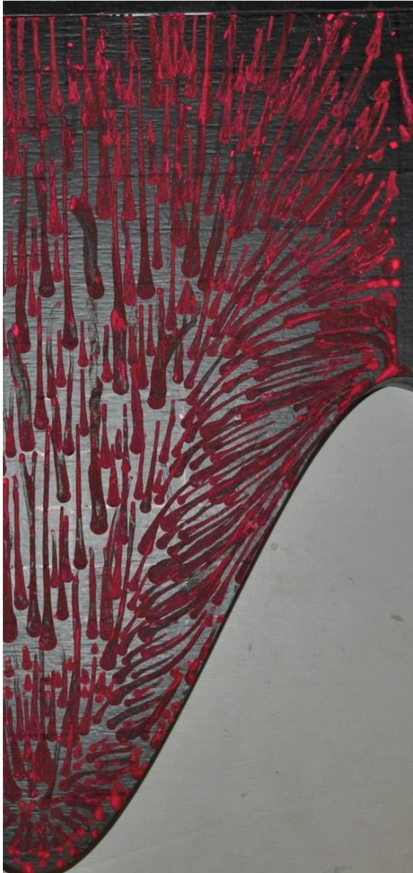
Figure 138: Surface shear stress visualisation over Sinusoidal FFS:  $A/\lambda = 0.65$ .
