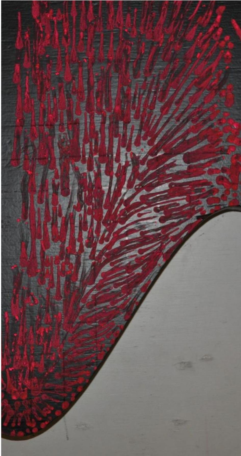
Figure 137: Surface shear stress visualisation over Sinusoidal FFS:  $A/\lambda = 0.5$ .
