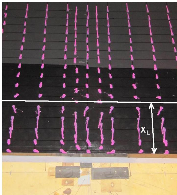
Figure 160: Boundary layer configuration 1,  $\delta/h = 1.35$ ,  $X_L/h = 2.375$ . Flow from bottom of photo to top.
