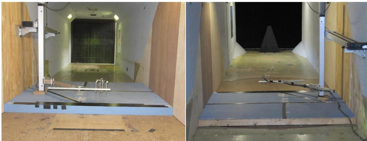
**Figure 43 (Left) View of straight edged FFS case from upstream. Note four Cobra Probes traversing. (Right) View of 0° straight edged FFS case from downstream. Note trapezoidal tooth trip to promote mixing.**
