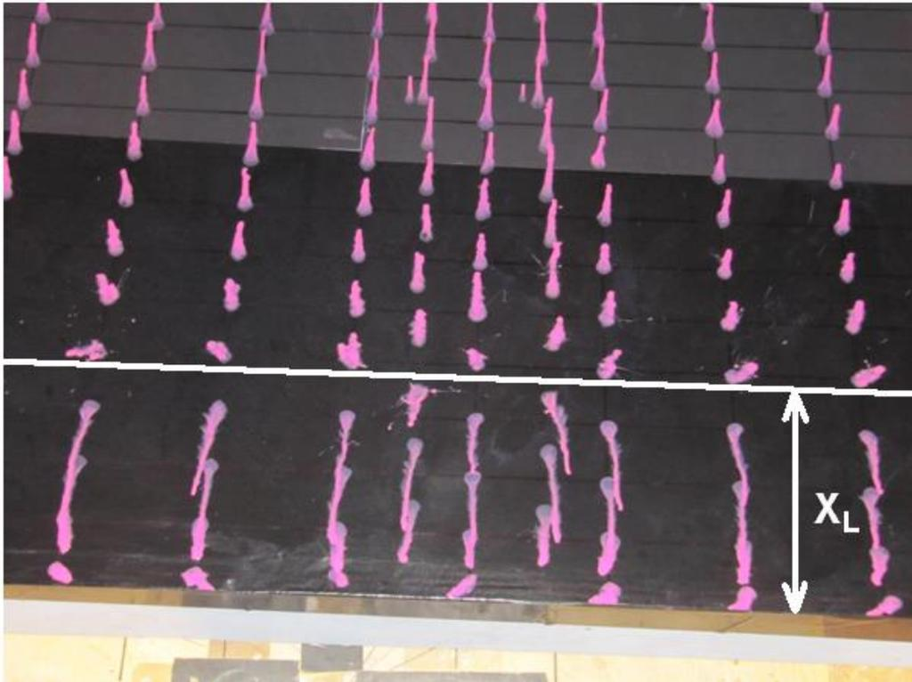
Figure 161: Boundary layer configuration 2,  $\delta/h = 7.15$ ,  $X_L/h = 1.9$ . Flow from bottom of photo to top.
