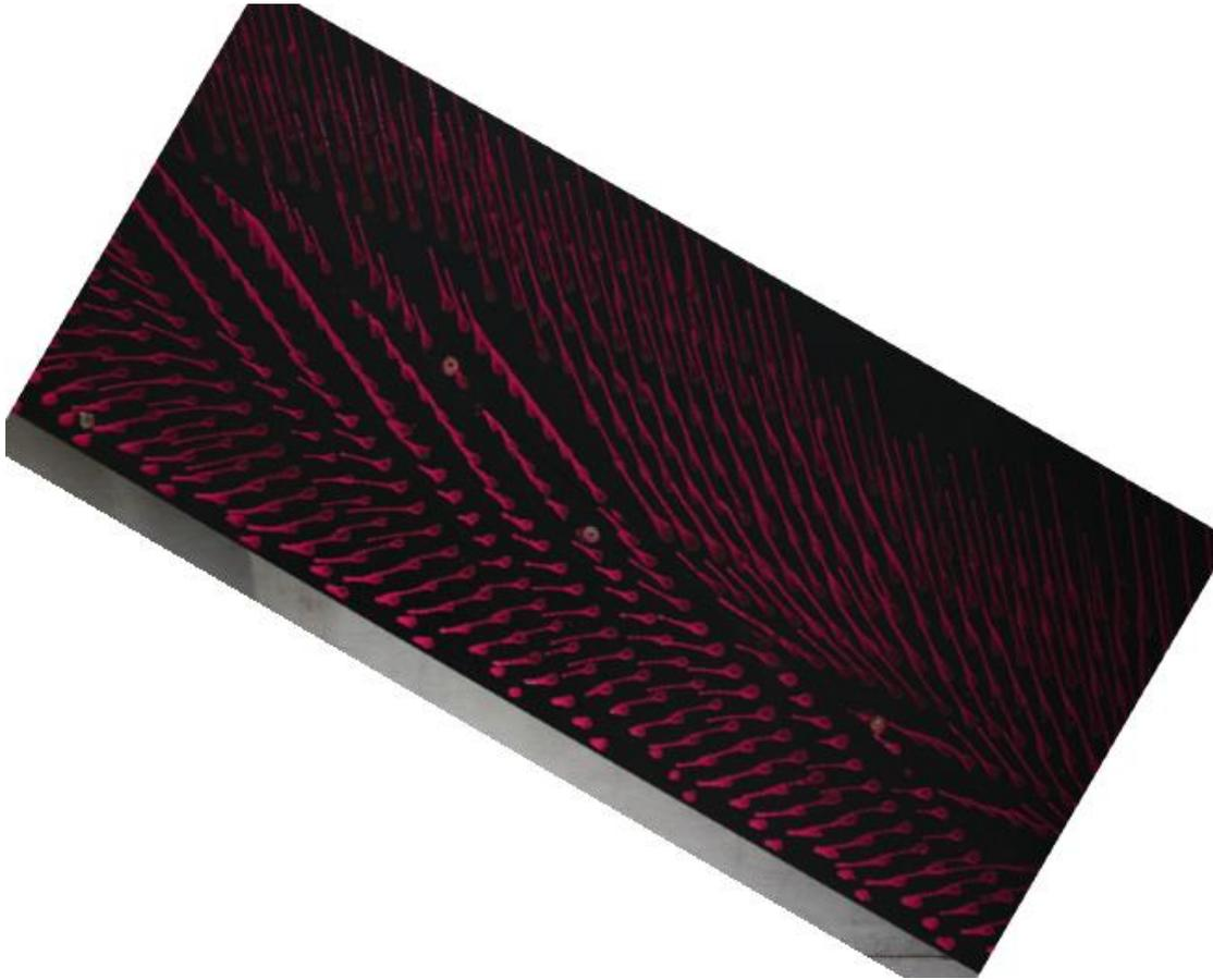
Figure 184: Paint droplet surface shear stress visualisation for  $\delta/h = 2$ . Yaw angle,  $\theta = 30^\circ$ . Inflow Configuration 3. Step height,  $h = 50$  mm. Flow direction from bottom of page to top.
