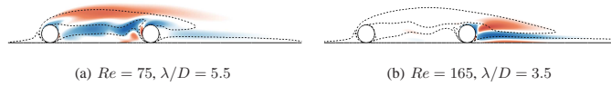
Figure 15: Spanwise perturbation vorticity for (a) the first and (b) the second transition to three-dimensionality for S/D = 5 . Contour shading as in figure 12.
