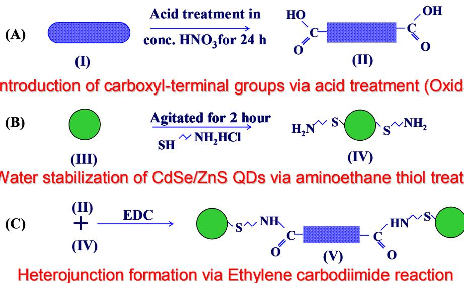
**Figure 1.** Schematic of the conjugation of MWCNTs to ZnS capped CdSe nanocrystals. (A) As grown MWCNTs (I) were oxidized by refluxing it in HNO<sub>3</sub> at 130 °C for 24 h to open the ends and create carboxylic group terminating MWCNTs (II). (B) ZnS capped CdSe QDs in chloroform (III) agitated with AET to stabilize them in aqueous PBS (IV). (C) Heterojunctions of CNT-QDs were synthesized by using a zero length cross linker EDC.
