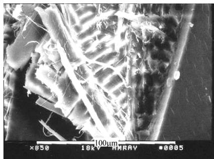
Fig.3. A helicoidal ply in elytra
