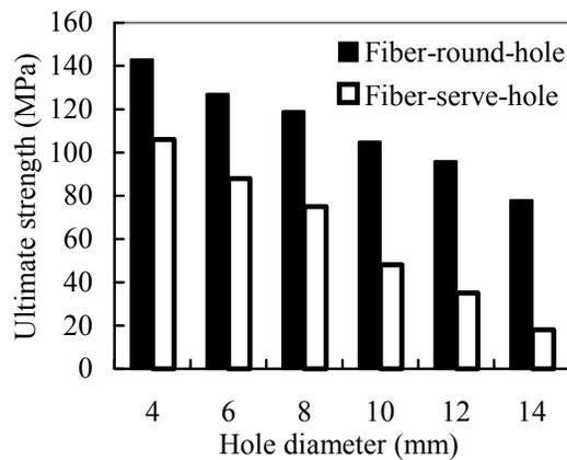
Fig. 7. The ultimate strength of the specimens with preformed and drilled holes
