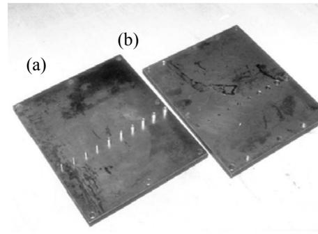
Fig. 6. (a). The bottom mould board containing circular pins of different diameter; (b). The upper mould board with matched holes
