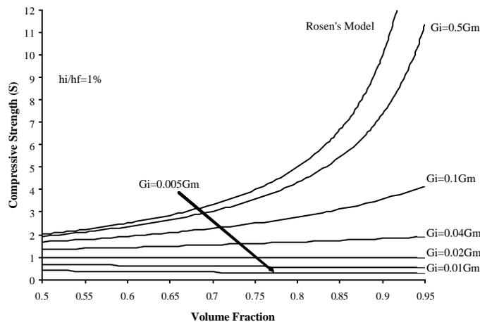
Fig. 2. Predicted compressive strength for various inter-phase moduli.
