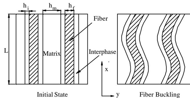
Fig. 1. Three-phase micro-buckling model.
