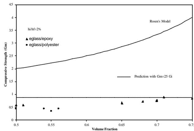
Fig. 5 Compressive strength of E-glass fiber composites (data from [23, 24]).
