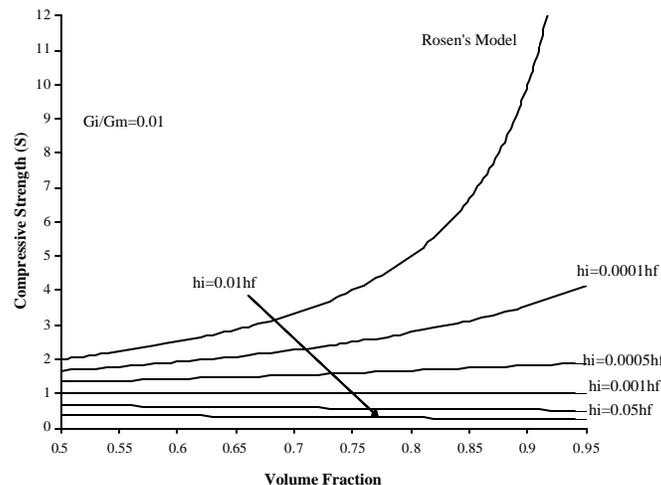
Fig. 3. Predicted compressive strength as a function of inter-phase thickness.
