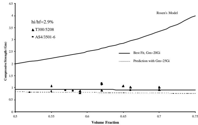
Fig. 4. Compressive strength of high strength carbon fiber composites (data from [23, 24]).
