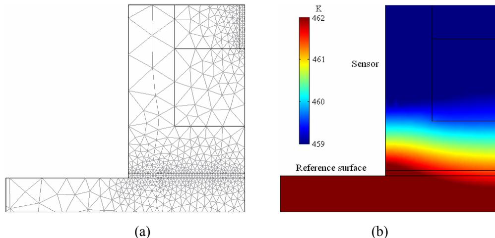
*Fig. 2. Numerical solution near the measuring section for one of the problems considered: (a) computational grid; (b) isotherms.*
