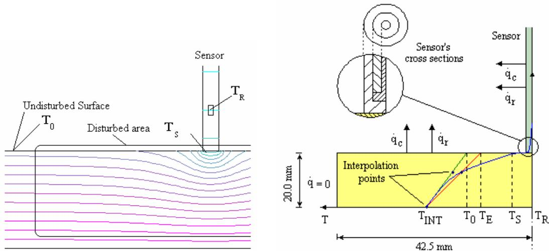
*Fig1. Sketch of temperature distribution in the calibration system with the sensor: (a) isotherms, (b) Computational domain and temperature along the sensors axis.*
