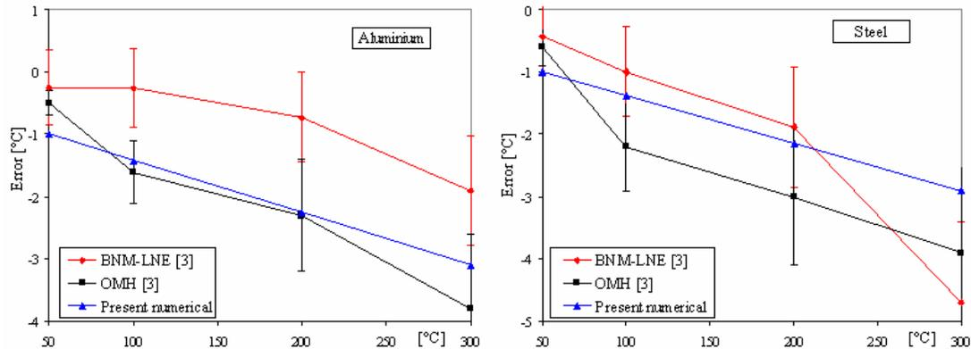
Fig. 3. Comparison of numerical and experimental results of the errors of the calibration system studied.
