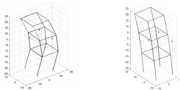
Figure 6 – Mode shapes of closely spaced frequencies identified with FDD method
