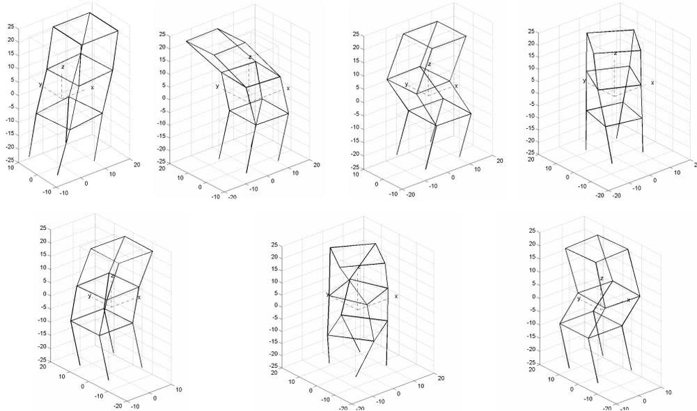
Figure 5 – Operational deflection shapes obtained with PP method
