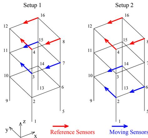
Figure 2 – Placement of accelerometers in each setup
