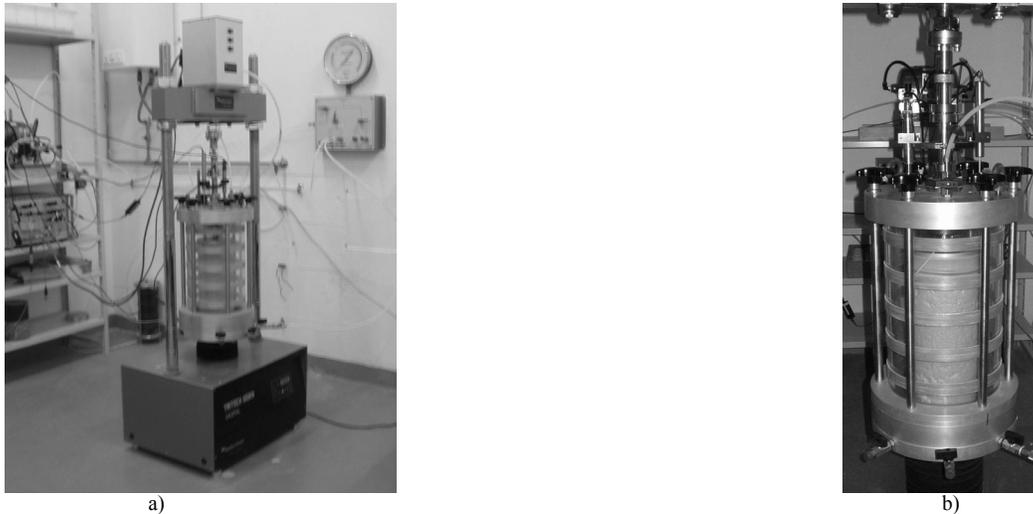
Figure 1- a) Tri-axial equipment of Lab of Road Pavement Mechanics of the Department of Civil Engineering of the University of Coimbra; b) Location of the LVDT's
