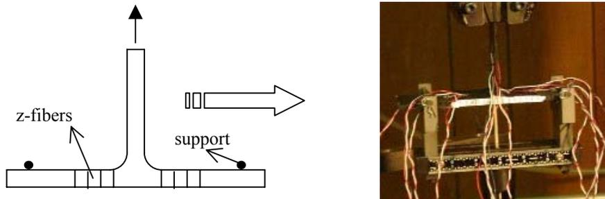
Figure 4. TPB test fixture.
