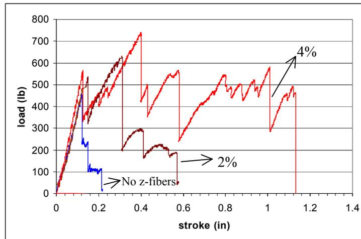
Figure 5. Load stroke readings of T-sections under TPB load.
