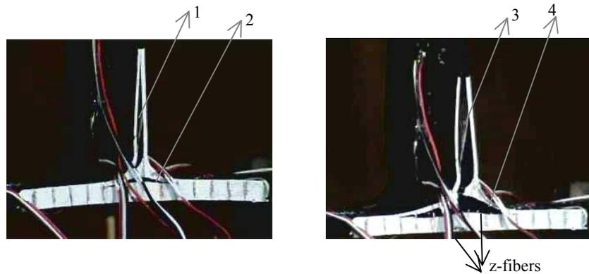
Figure 7. Delamination growth in T-section with z-fibers.
