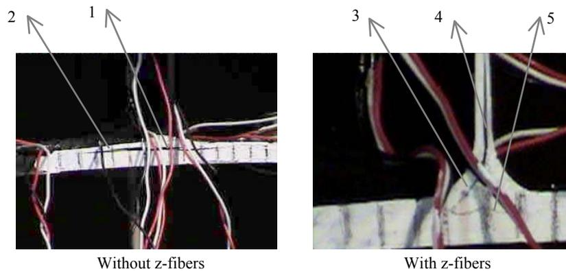
Figure 6. Delamination mechanisms in T-sections with and without z-fibers.
