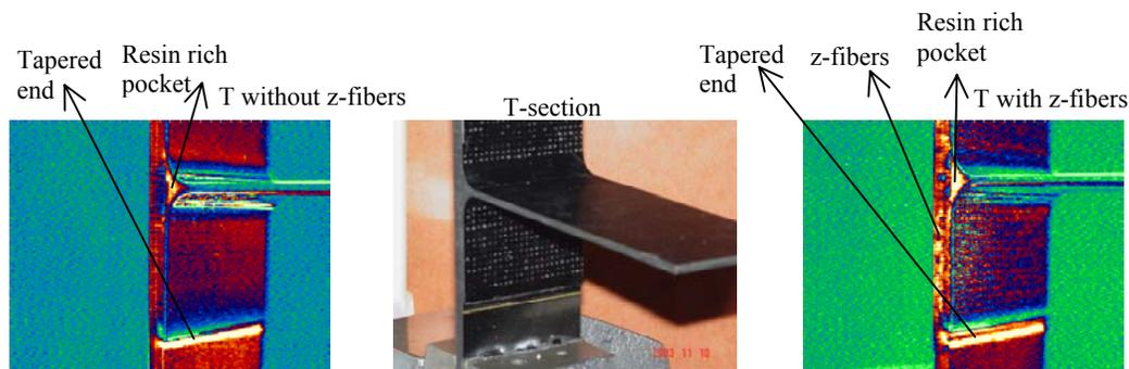
Figure 3. TSA pictures from infrared camera.
