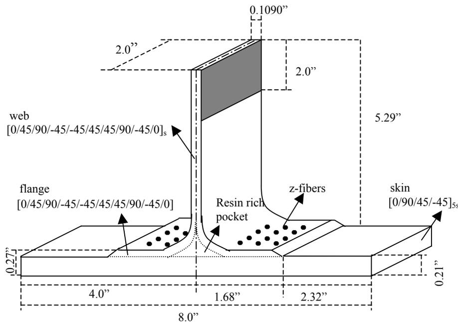
Figure 1. Specimen dimensions and lay-ups.
