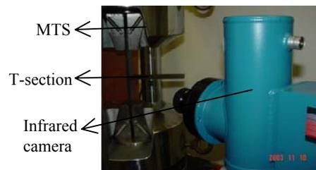
Figure 2. TSA test set-up.
