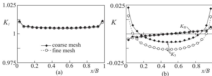
Figure 3: Stress intensity factors (a)  $K_I$ , (b)  $K_{II}$  and  $K_3$ .
