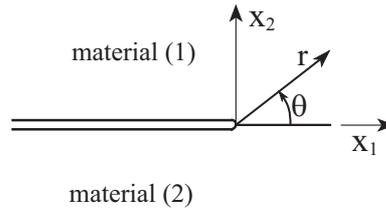
Figure 1: Crack tip coordinates.
