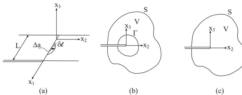
Figure 2: (a) Virtual crack extension  $\delta\ell$  for through crack. (b) In-plane volume  $V$ , outer surface  $S$  and inner surface  $\Gamma$ . (c) Inner surface  $\Gamma$  collapses to crack front.
