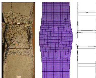
Figure 4: Comparison of experiment (left) and FE model. Damage zone with buckled reinforcement.
