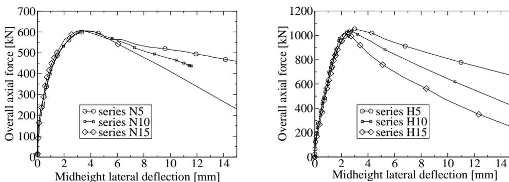
Figure 3: Experiments: Force vs. midheight lateral deflection diagrams of N (top) and H (bottom) series. Numbers 5, 10 and 15 stand for distance of stirrups in cm.
