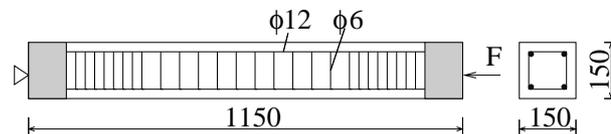
Figure 1: Geometry of specimens in mm (drawn in horizontal position).
