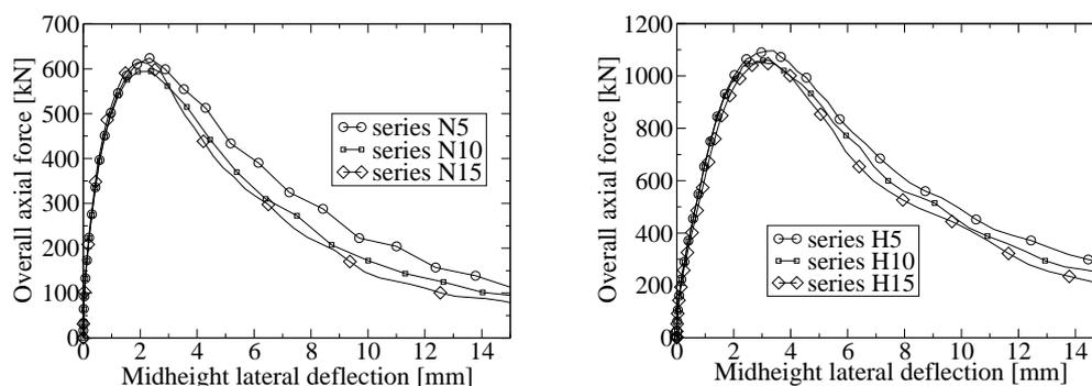
Figure 5: Simulation: Force vs. midheight lateral deflection diagrams of N (top) and H (bottom) series. Numbers 5, 10 and 15 stand for distance of stirrups in cm.
