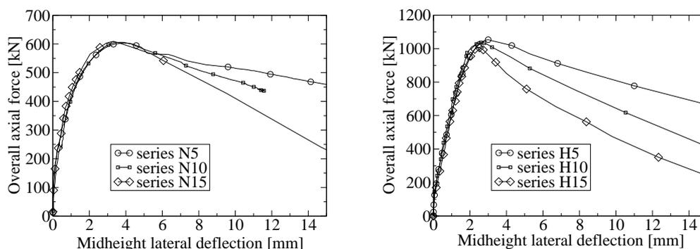
Figure 3: Experiments: Force vs. midheight lateral deflection diagrams of N (top) and H (bottom) series. Numbers 5, 10 and 15 stand for distance of stirrups in cm.
