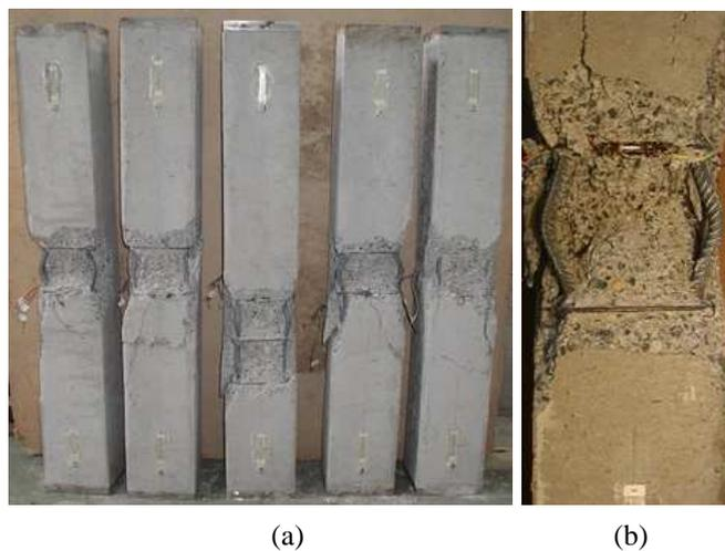
Figure 2: Experiments: (a) Series N10 after collapse. (b) Front view on the damaged zone at the midheight.
