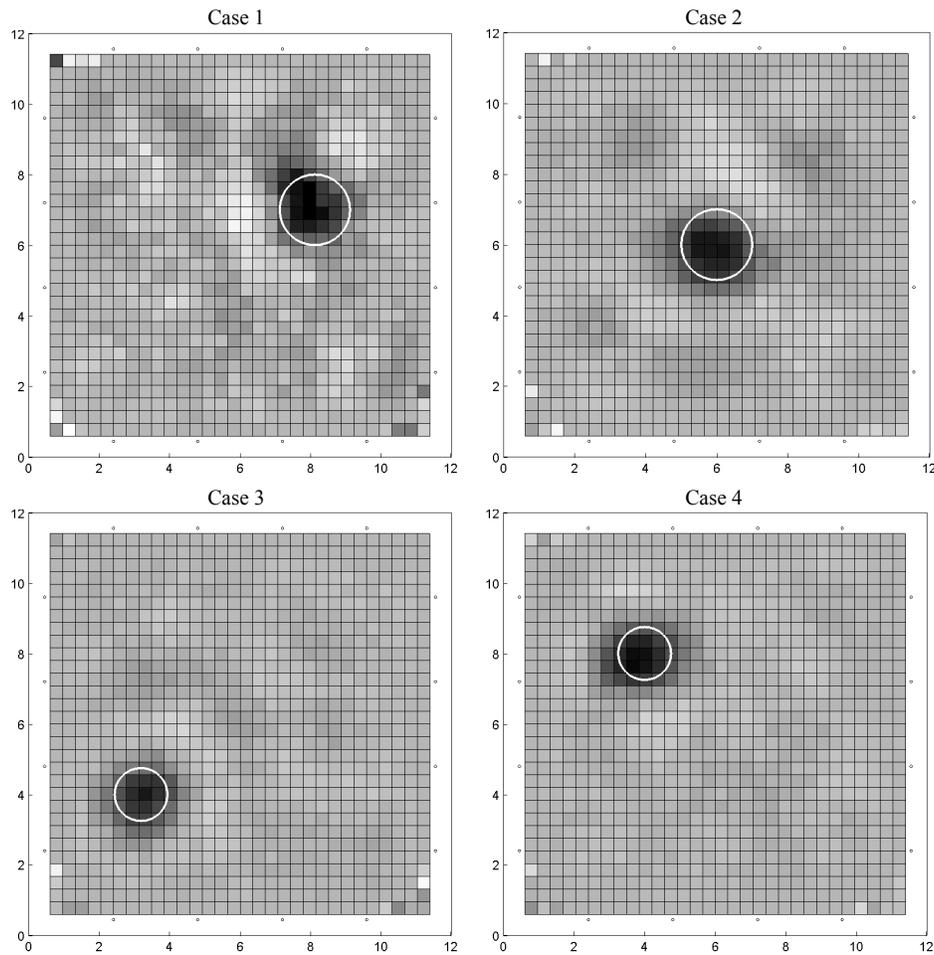
**Figure 2. Damage results for cell grid representation. The white circle indicates the actual damage. Results range from 1.4 (white) to 0 (black).**
