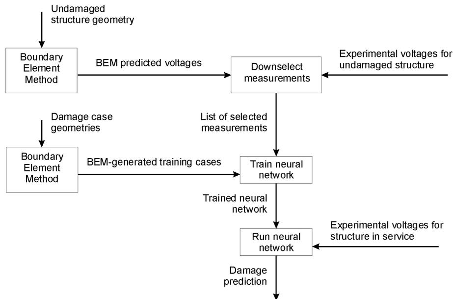
Figure 1. Flowchart of damage detection process.
