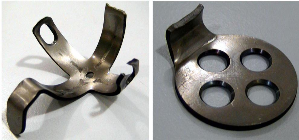
Figure 5 – Fracture of an ARD after testing.
