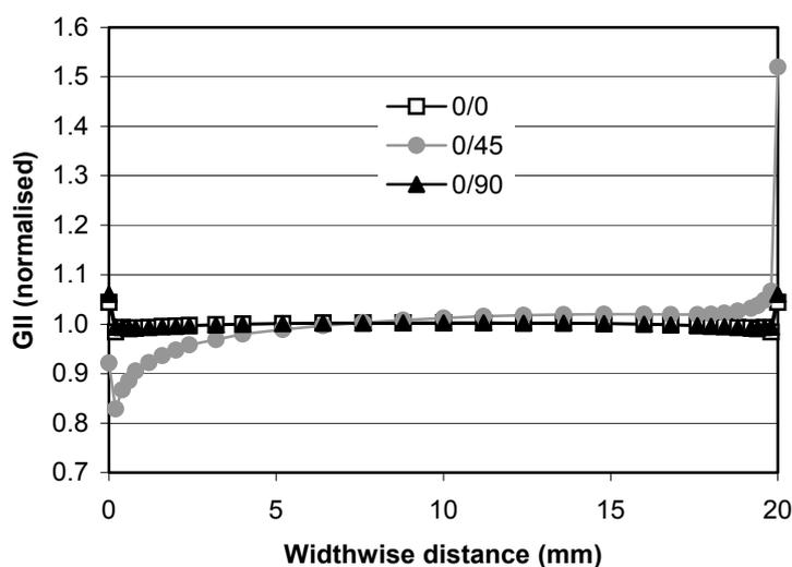
Figure 2. Distributions of  $G_{II}$  along the width of ENF specimens.  $G_{II}$  values were normalised by the widthwise average.
