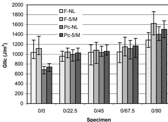
Figure 3. Average  $G_{IIc}$  and scatter range obtained from the film (F) and precrack (Pc) using the non-linearity (NL) and the 5 % offset or maximum load (5/M) criteria.
