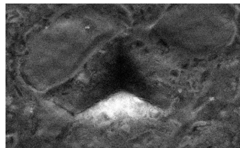
Figure 2. Indent in CSH gel (sample after heating to 800 °C).
