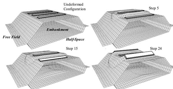
**Figure 1:** Deformed configurations of BIRF of ground-tie system at selected times
