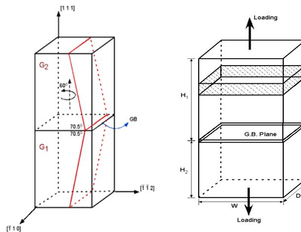
**Fig 1.** Schematic of the Nanospecimen
