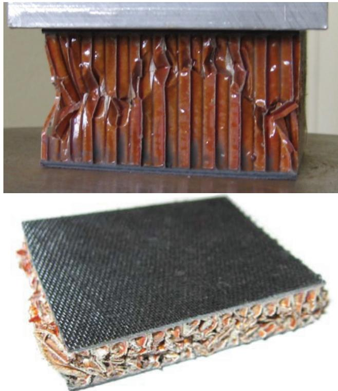
Figure 2: Shapes of failure of an ECA-R specimen during and after compressive loading
