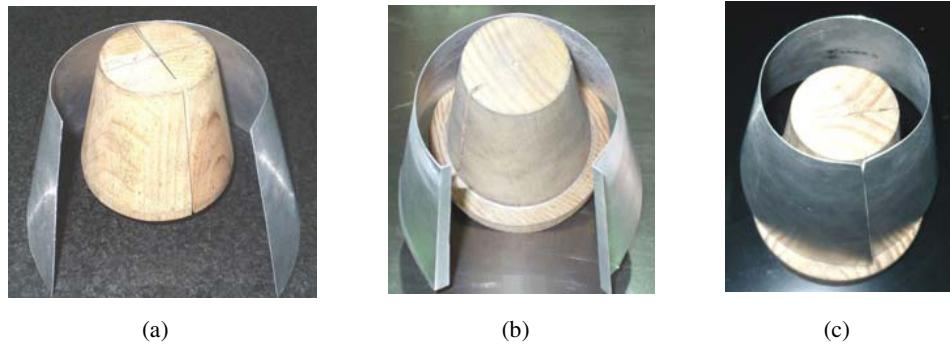
Figure 3: Aluminum sheet truncated cones molded with wood truncated cones
