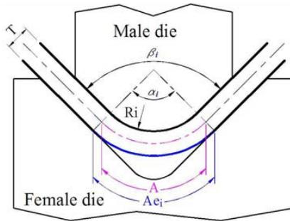
Figure 1: The bending process of metallic sheet (seated)
