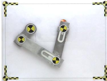
Figure 2: The four-bar prototype
