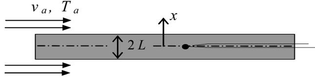
Figure 1: Scheme of the drying experiment
