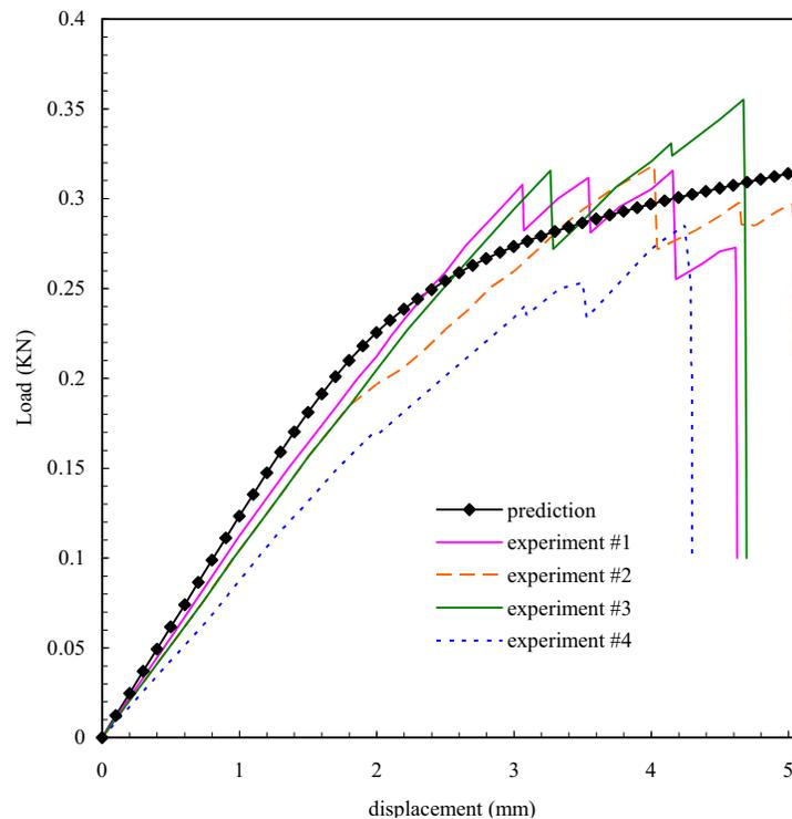
Figure 1: The comparison of load-displacement curves between the present prediction and experimental data[12] under three-point bending[9]
