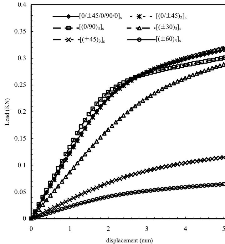
Figure 2: The load-displacement curves of laminated composite beam with various stacking sequence
