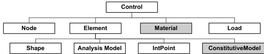
Figure 1: Classes hierarchy of FE computer system
