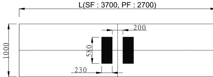
Figure 2: Position of load application
