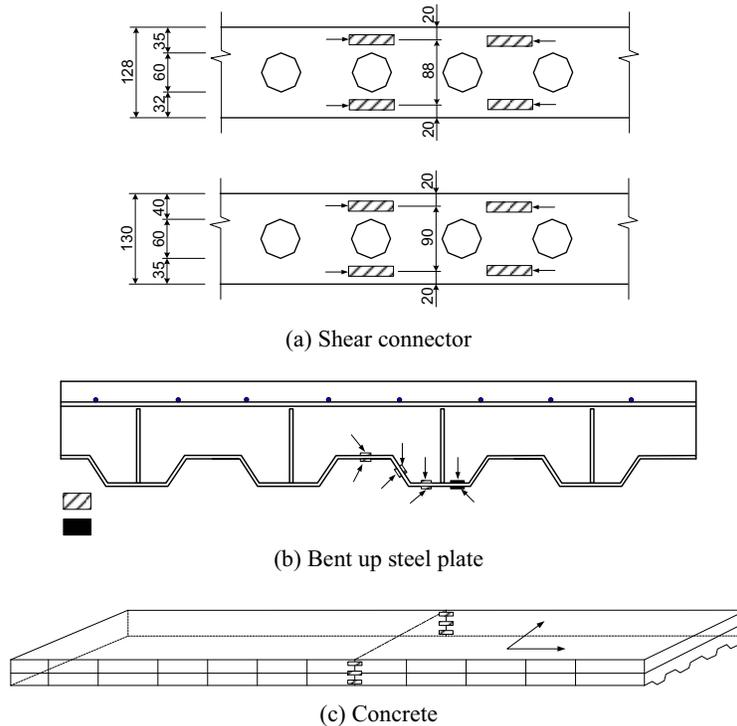
Figure 1: Attachment positions of strain gauge
