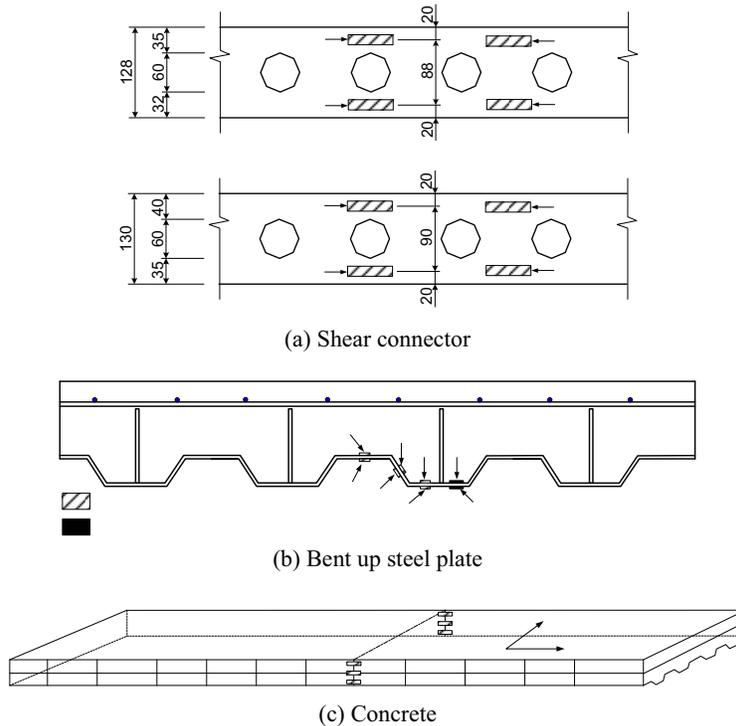
Figure 1: Attachment positions of strain gauge
