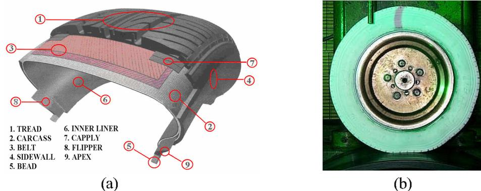
Figure 1: Radial tire. (a) structural composition, (b) standing wave experiment.
