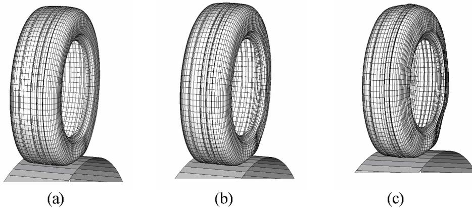
Figure 5: Simple model (type A). (a) 160km/h, (b) 205km/h, (c) 245km/h.
