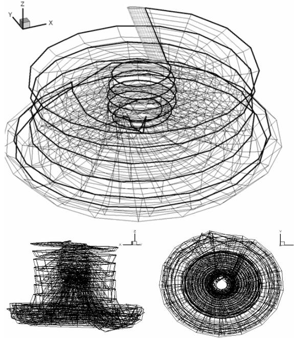
Figure 4: Wake geometry in the hovering with 1-blade
