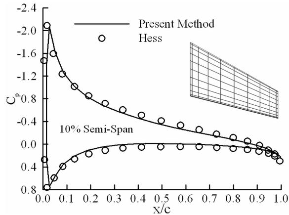
Figure 3: Pressure distribution of the thin swept blade
