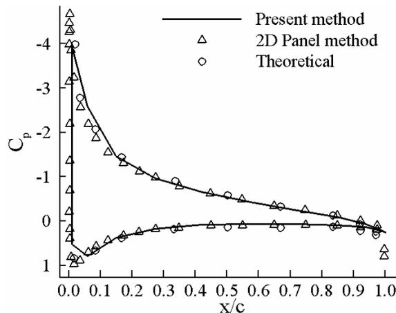
Figure 2: Pressure distribution of NACA 0012 at the AOA=8.3
