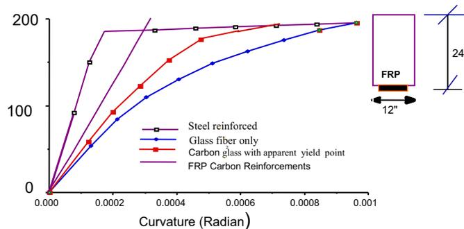
Figure 2: Moment Curvature Behavior of Fiber Material
