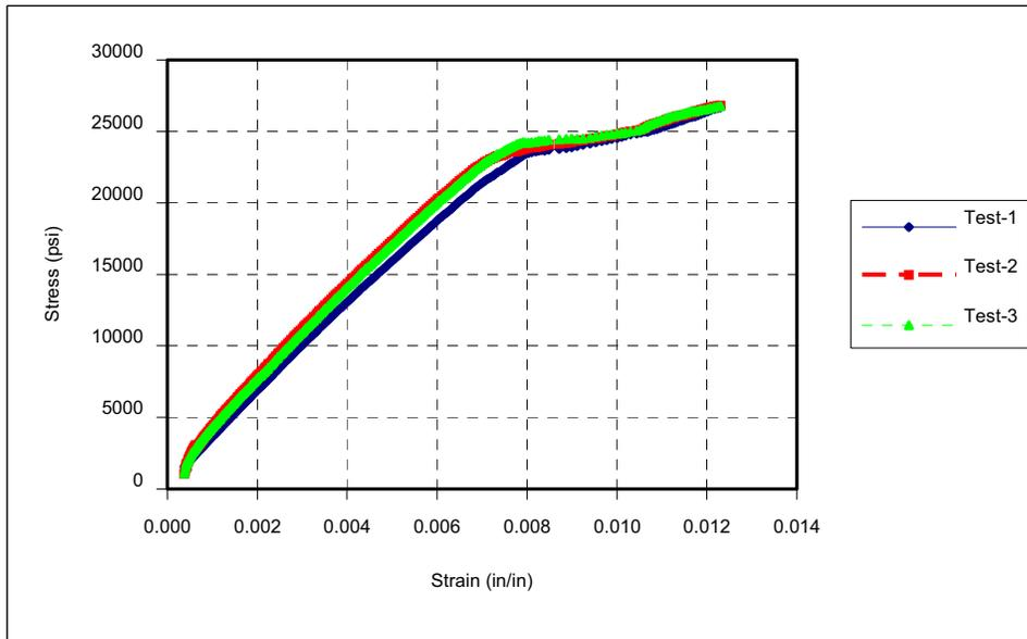
Figure 1: Stress strain plots for Set 4 with an apparent yield point.
